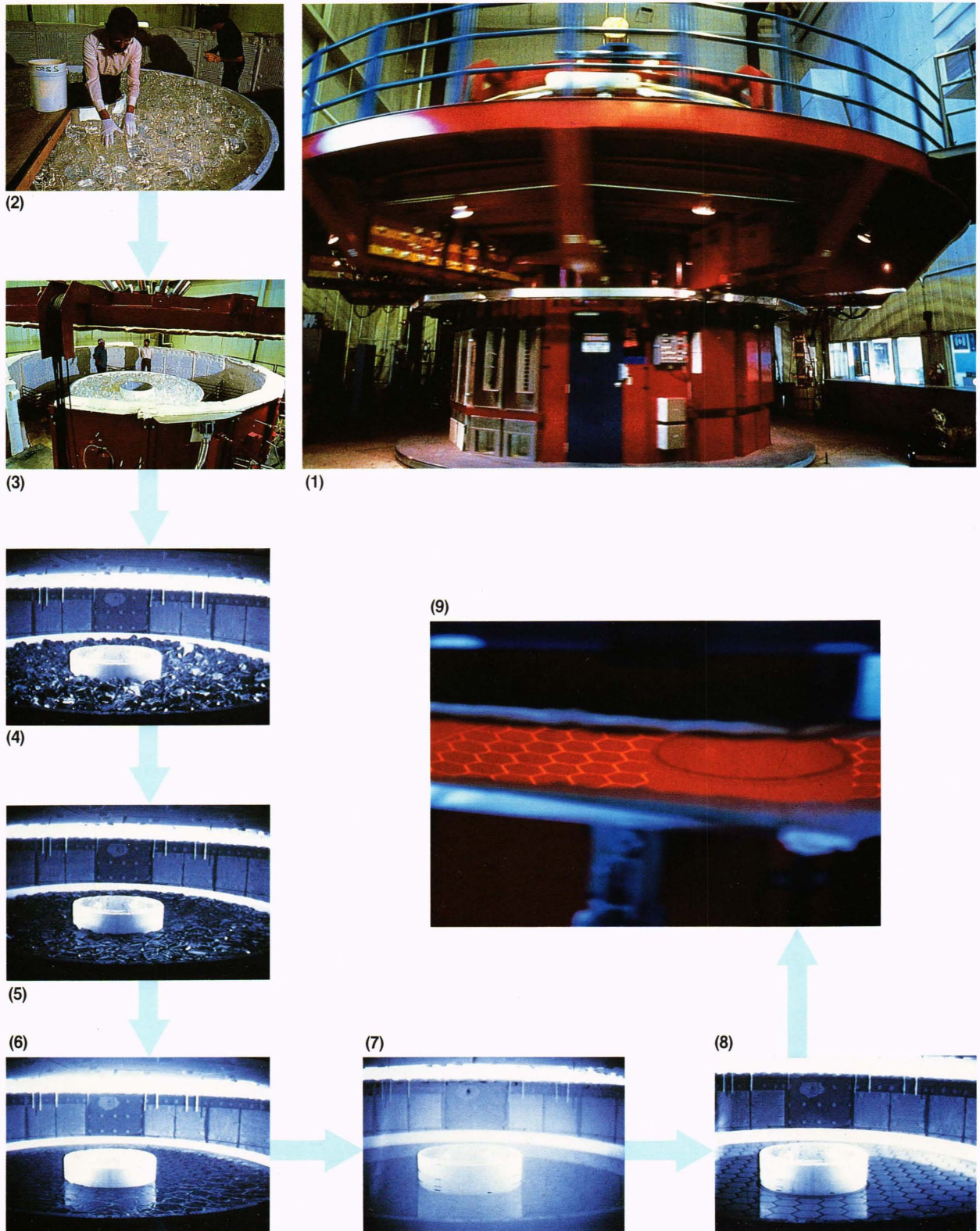
Figure 3 —This dramatic sequence of photographs, taken in April 1988, shows the stages in the manufacture of a spin-cast 3.5-m mirror. The furnace (1) in which the mirror is made resembles a carousel. In the sequence, we see the chunks of borosilicate glass being loaded into the furnace (2) and the glass before closing the lid (3). Note the capacity of the furnace to make mirrors with diameters up to 8 m. As the furnace temperature increases from 829°C (4) through 907°C (5) to 960°C (6), the glass melts into a liquid mass. Spinning begins at 1170°C (7), and the glass forms the paraboloidal shape. Note the increased height of the central shape as the dish forms and the rib structure visible through the mirror surface. After cooling has allowed the glass to harden (8), the furnace lid is cracked (9) to show the still red-hot mirror. (Photographs courtesy of Roger Angel, University of Arizona Mirror Laboratory.)
