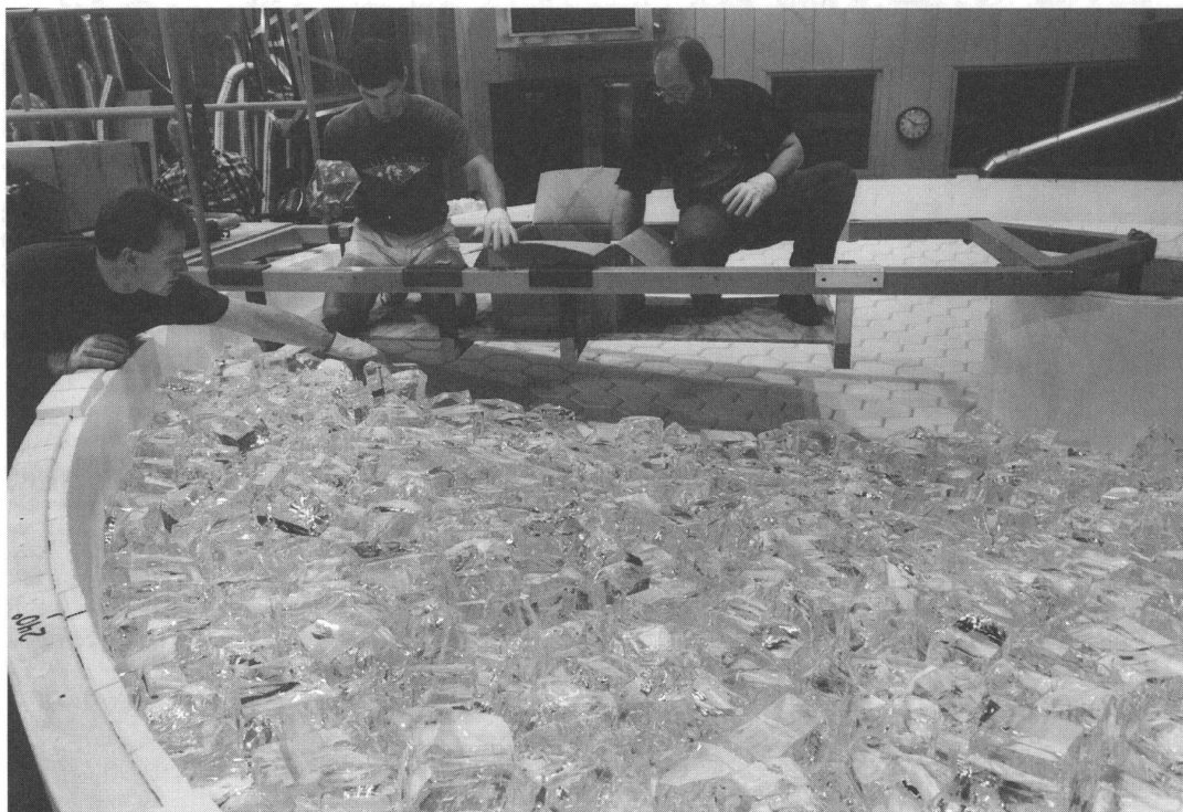
Figure 6: This photo shows Mirror Lab technicians Warner, Lutz and Watson loading chunks of E6 borosilicate glass into the honeycomb mold. The glass must be carefully loaded by hand to avoid damaging the friable honeycomb mold. 9550 kg of glass was loaded into the mold. UA photo by Lori Stiles
