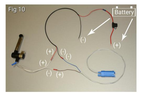
Alternatively, a connection/junction box can be used, the connections can be seen below. (1)
