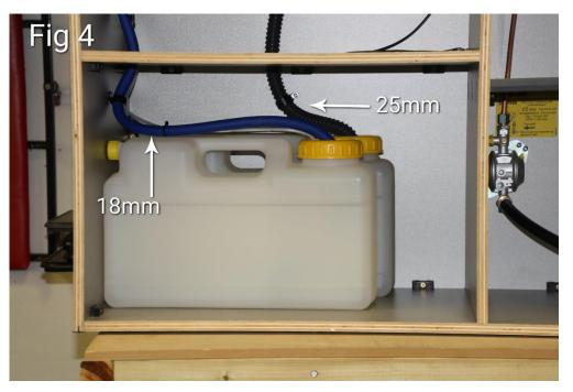
The route for the waste pipe can be either directed into an onboard waste container the same size as the fresh water container (Stored with in the internal cupboards of the van), often used in removable Pod Units. ④ Alternately, the waste pipe can be taken externally through the floor of the van, this would end with a short tail under the van that could then be directed into a portable waste container as is needed. ⑤
