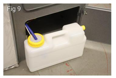
Ensure that the water pipe is long enough to allow the water container to be completely removed from of the storage cupboard. (9) If you fail to allow this in the pipe length then it will be difficult to remove the water container from the cupboard, and even harder to re-install it once it has been filled with water.
