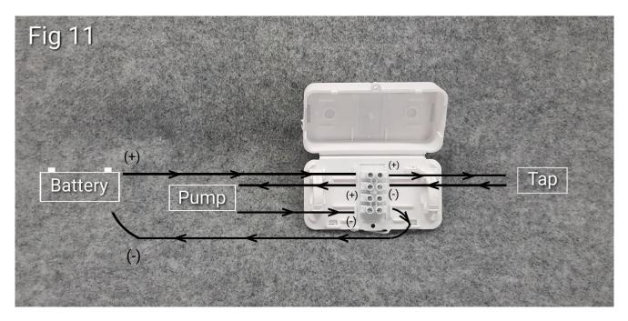
The wiring diagram above shows a basic looping circuit with the tap operating as an inline switch. When the tap lever is lifted the circuit is completed allowing the pump to activate.
