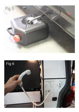
The final option for waste water storage is to take the waste pipe through the floor and into a waste tank fitted underneath the vehicle. This is usually only suitable for larger van conversions or motorhomes. Or when there is a specific need to carry a larger water capacity, for example if you plan to fit a shower 6
