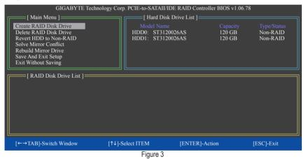
**Note:** In the main screen, you can select a hard drive in the **Hard Disk Drive List** block and press <Enter> to see detailed information about the selected hard drive.
