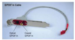
1. Installing the S/PDIF In Cable:
