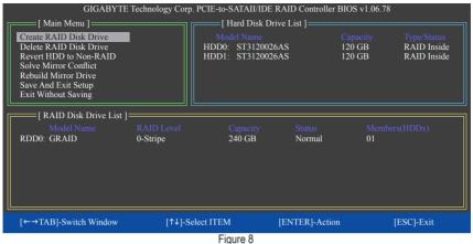
To check more detailed information about the array, use the <Tab> key while in the **Main Menu** block to move the selection bar to the **RAID Disk Drive List** block. Select the array and press <Enter>. A small window displaying the array information will appear in the center of the screen (Figure 9).
