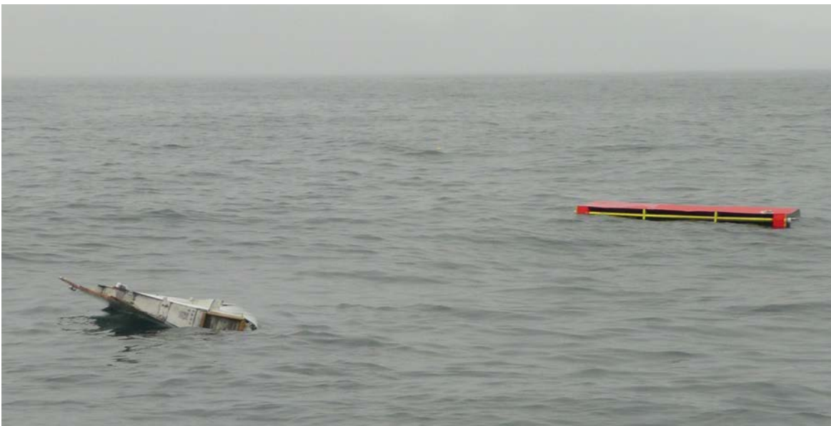
Fig. 1.3 Genuine (left) and replica (right) flaperons at sea in calm weather during field measurements of their rate of drift through the water. Water movement was monitored using GPS-equipped buoys.
