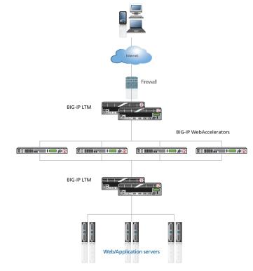
Figure 1: Configuration example
