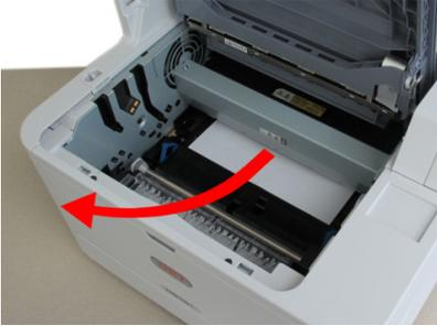
6. Lower the top cover but do not press down to latch it closed yet. This will protect the drum from excessive exposure to room lighting, while you check the remaining area for jammed sheets.
