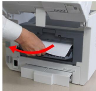
**NOTE:** Check that there is no paper remaining inside the machine. Remove the paper carefully so that it does not tear. If the paper tears, be sure to remove all of the pieces.
