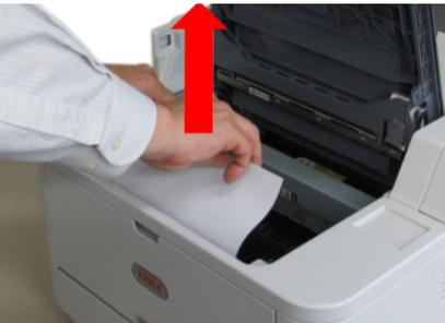
8. Remove any paper from the rear of the printer.
