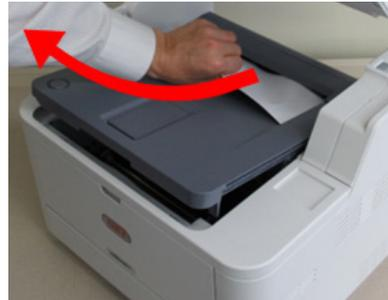
To remove paper when the bottom edge of the paper is visible.
