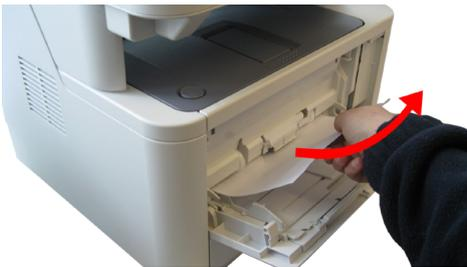
NOTE: If you have failed to remove jammed paper do not use force to pull out the paper but follow the steps below.
