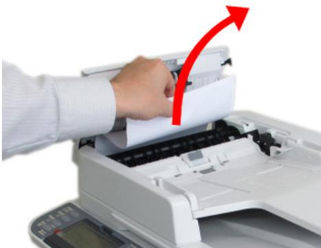
3. If the edge of the document can be seen under the paper guide. Lift up the guide (1) and gently remove the jammed paper (2).
