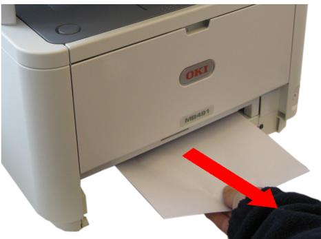
After successful removal of any damaged or misfed paper, the printer should continue printing.
