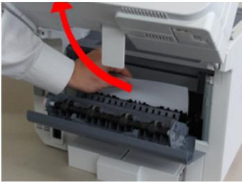
If you are not using the rear cover, close it once the paper has been removed from this area.
