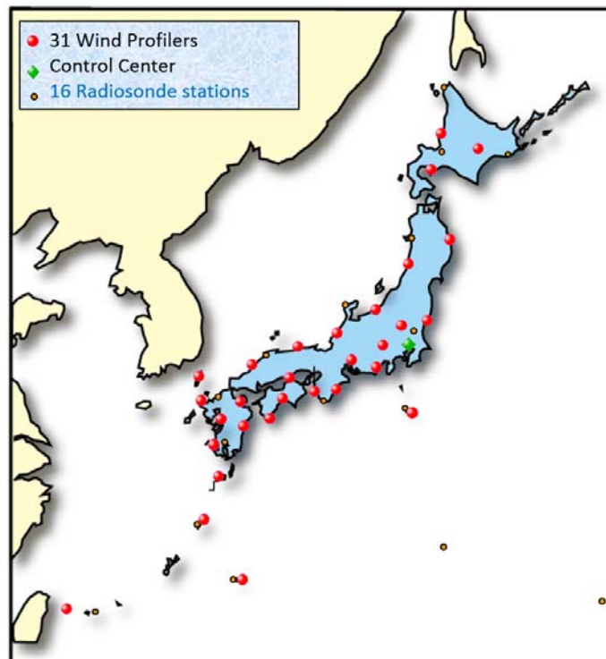
Fig. C-1-1. Upper air observation network of JMA. Large red circles indicate wind profilers, and small orange circles show radiosonde stations. After Saito et al. (2015).
