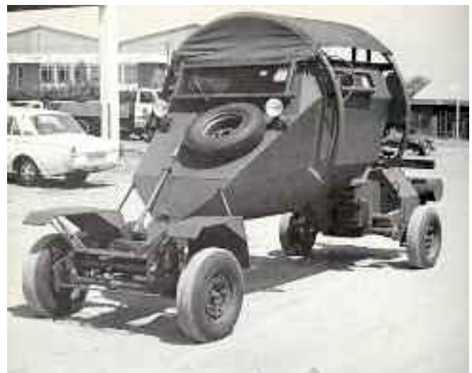
Figure 6. The Leopard. It incorporated the V-shaped hull with the single monocoque hull which provided protection to the drive-train as well as the passenger compartment. The increased axle length brought the wheels outside the passenger compartment and the easily sheared connection meant that the wheel assembly would be blown clear of the vehicle if it detonated a mine. (Source: Ernest Konschel. Available from: http://www.baragwanath.co.za/leopard/ )
