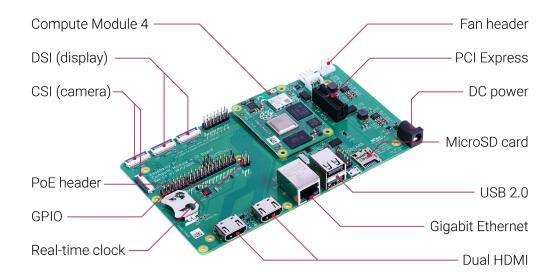
**Input power:** 12V input, +5V input with reduced functionality
