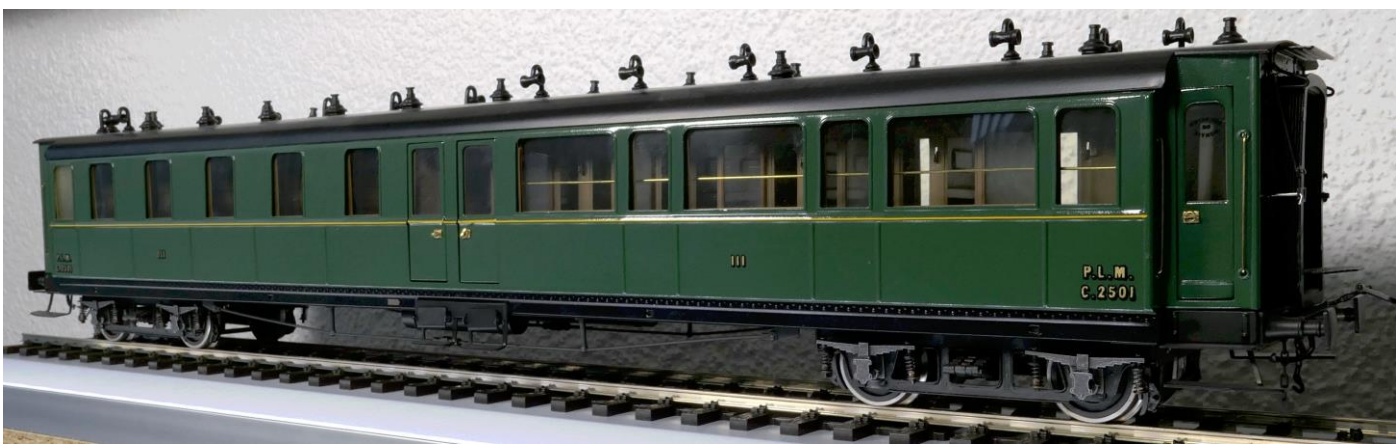
The all-green third-class car has what is called a Z-layout; The corridor switches positions with the compartments in the middle of the car. Each half has 5 compartments so a total of ten third class compartments is present. This car is the longest, the Elettren model is 52 cm long. As can be seen there are also doors in the centre of the car with folding steps below.
