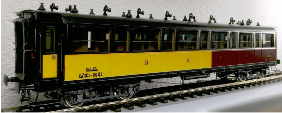
The first/second class car is peculiar with its two-colour livery. The picture shows it from the corridor side. It is an A3 B4 type car which means it has three first class and four second class compartments. The model is 44 cm long.
