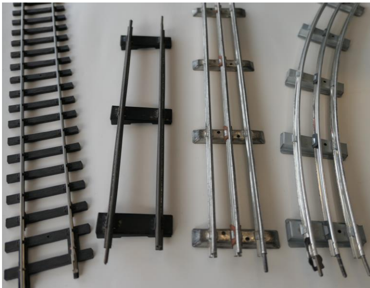
From left to right: Scale 2-rail rail from RivaRossi, Rossignol clockwork rail, tinplate 3-rail electric Merkur rail and a curve of JEP 3-rail electric tinplate rail.
