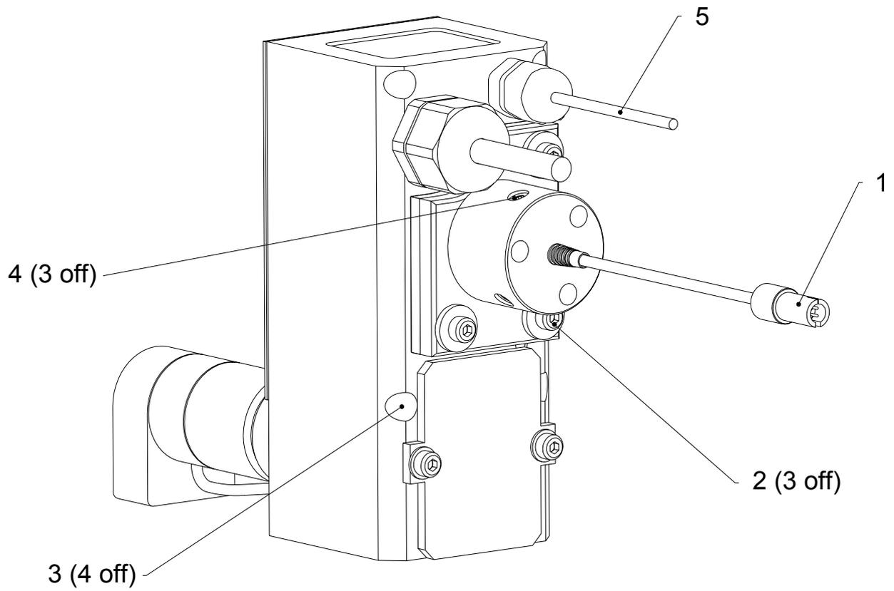
Figure 33 – Pointing Diode
