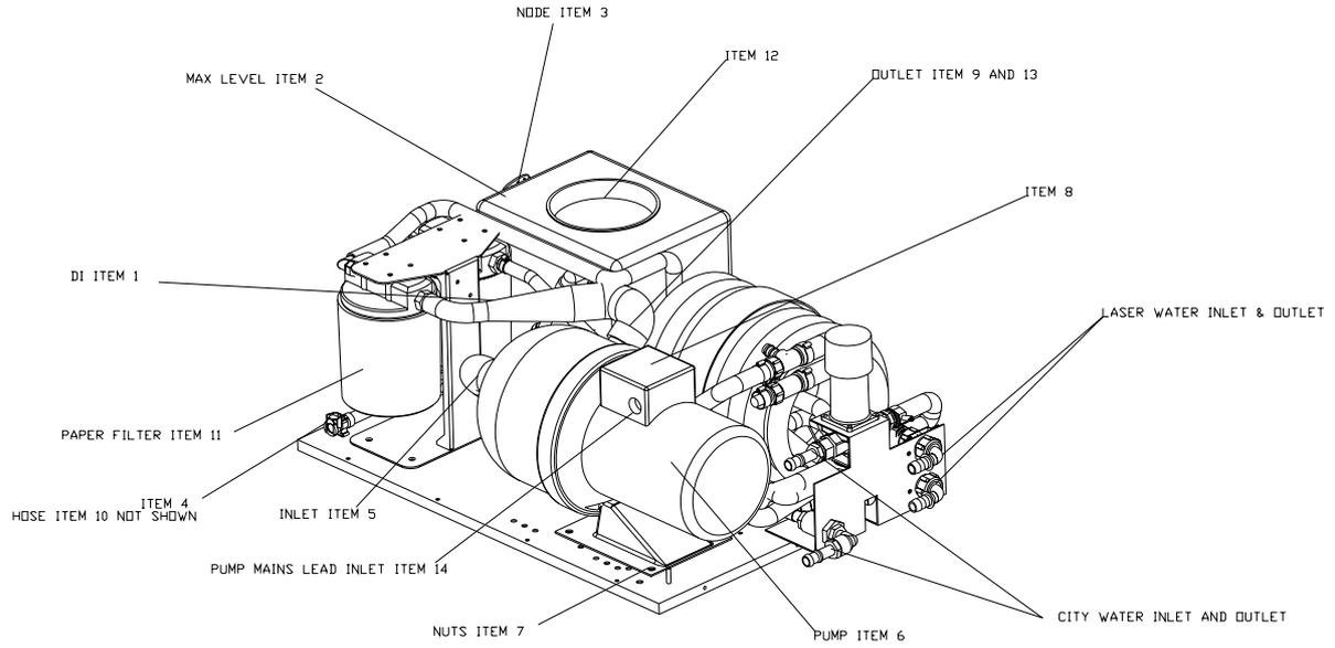
**Figure 18 – Coolant Pump Installation**
