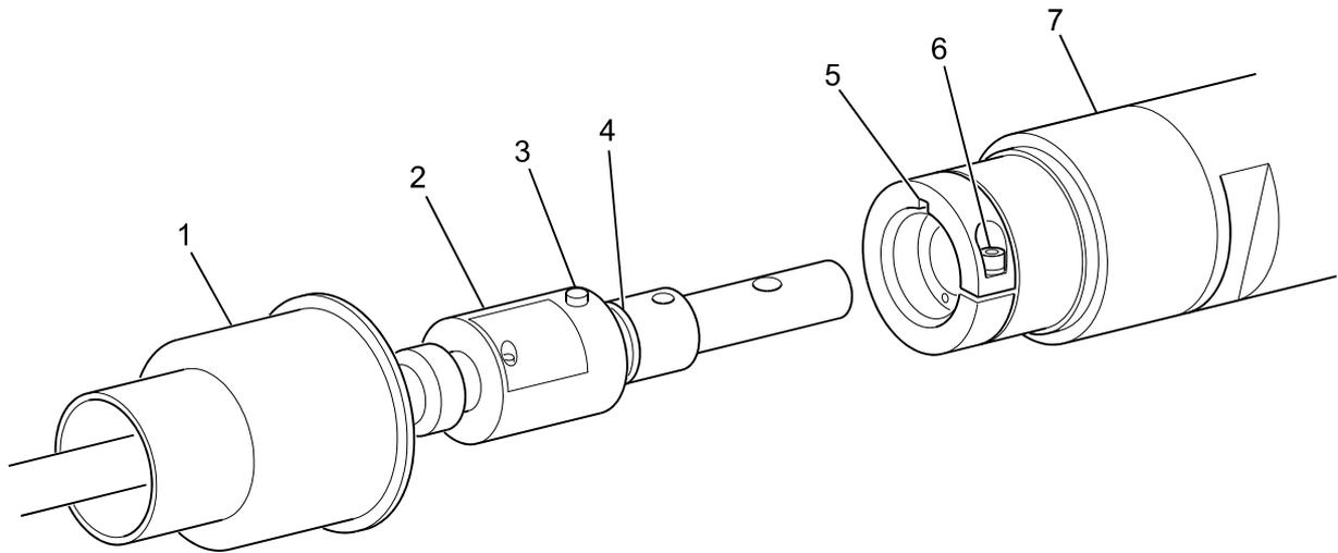
Figure 23 – Fibre Output Termination
