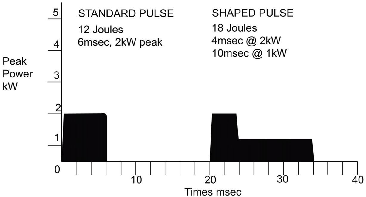
**Figure 34 - Basic laser pulse and shaped pulse**
