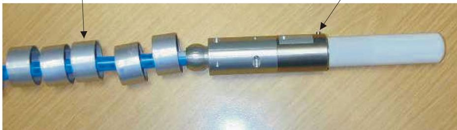
5. Build up the Bendlock assembly using the split-rings, sleeve and snap ring
