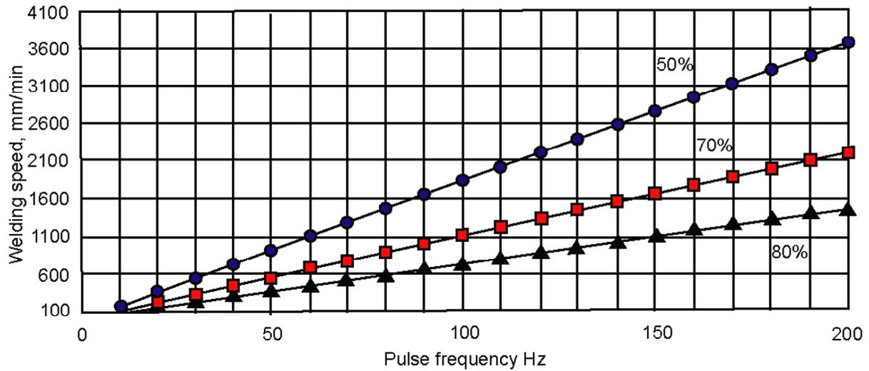
**Figure 35 – Welding speed vs repetition rate for different percent overlaps (spot size 0.60mm)**
