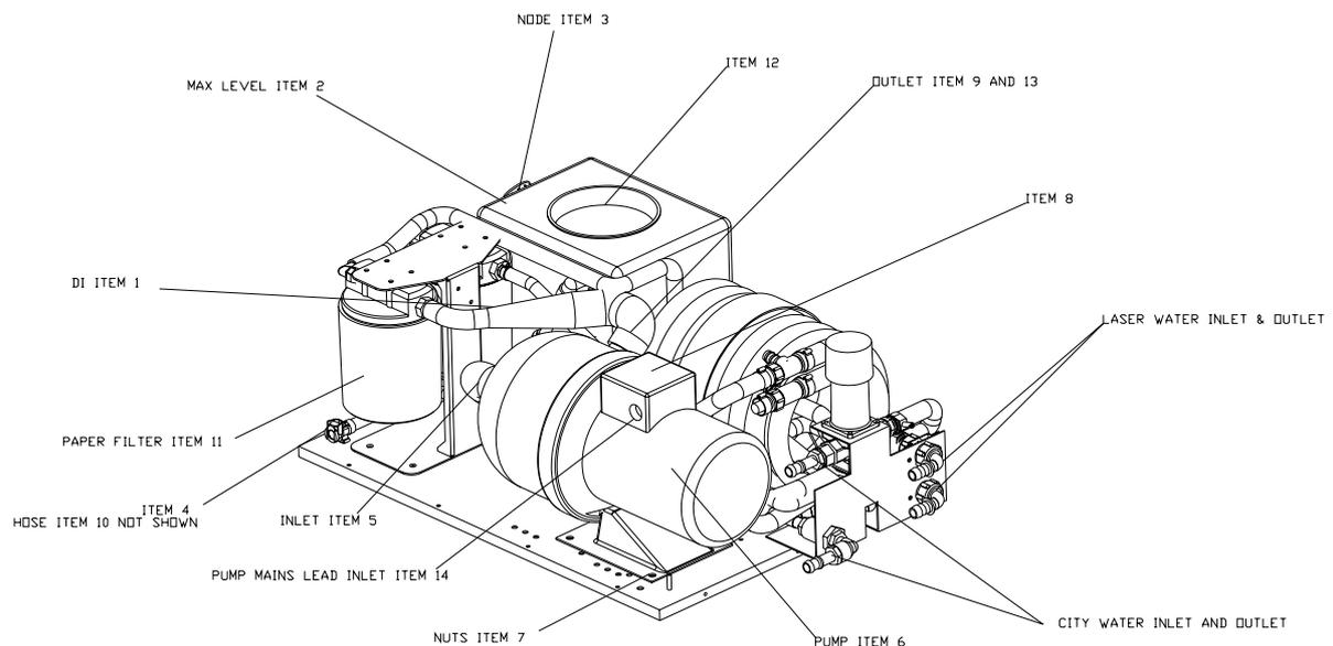
Figure 17 – Coolant Pump Removal
