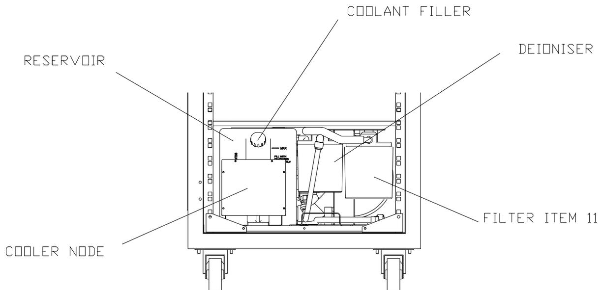
**Figure 13 – Coolant Draining**
