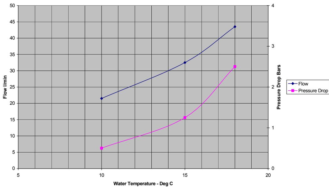
Figure 2 - External Water Parameters
