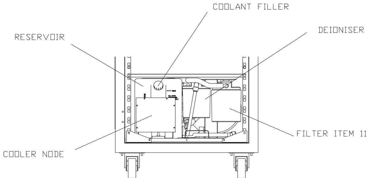
Figure 16 - De-ioniser Replacement Procedure
