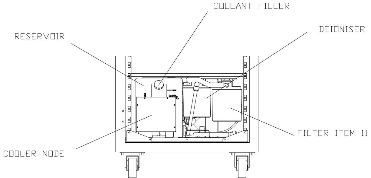
**Figure 14 – Coolant Filling**
