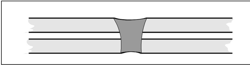
**Figure 37 – Undercut Overlap Weld**
