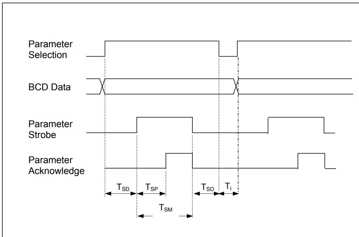
Figure 4 - Parameter Timing Diagram
