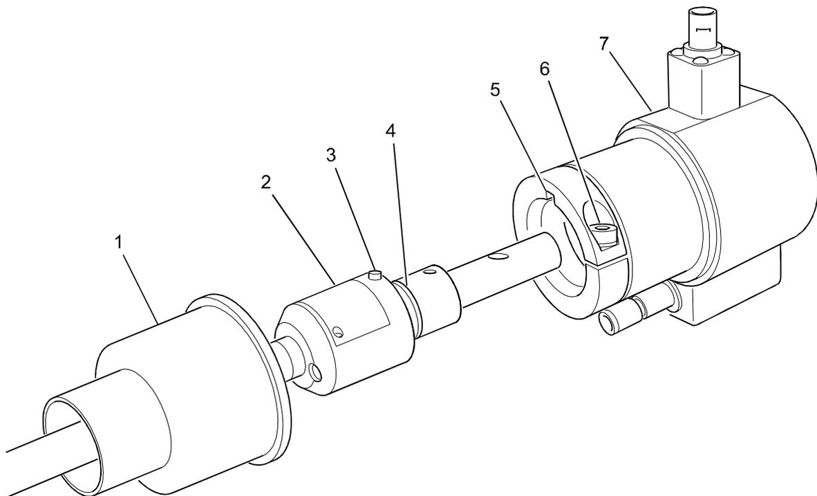
Figure 21 – PIPA Fibre Cable Removal
