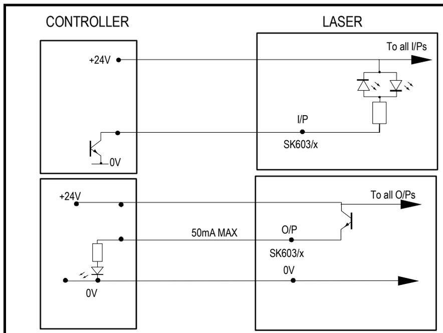
**Figure 9 - Sinking Diagram**
