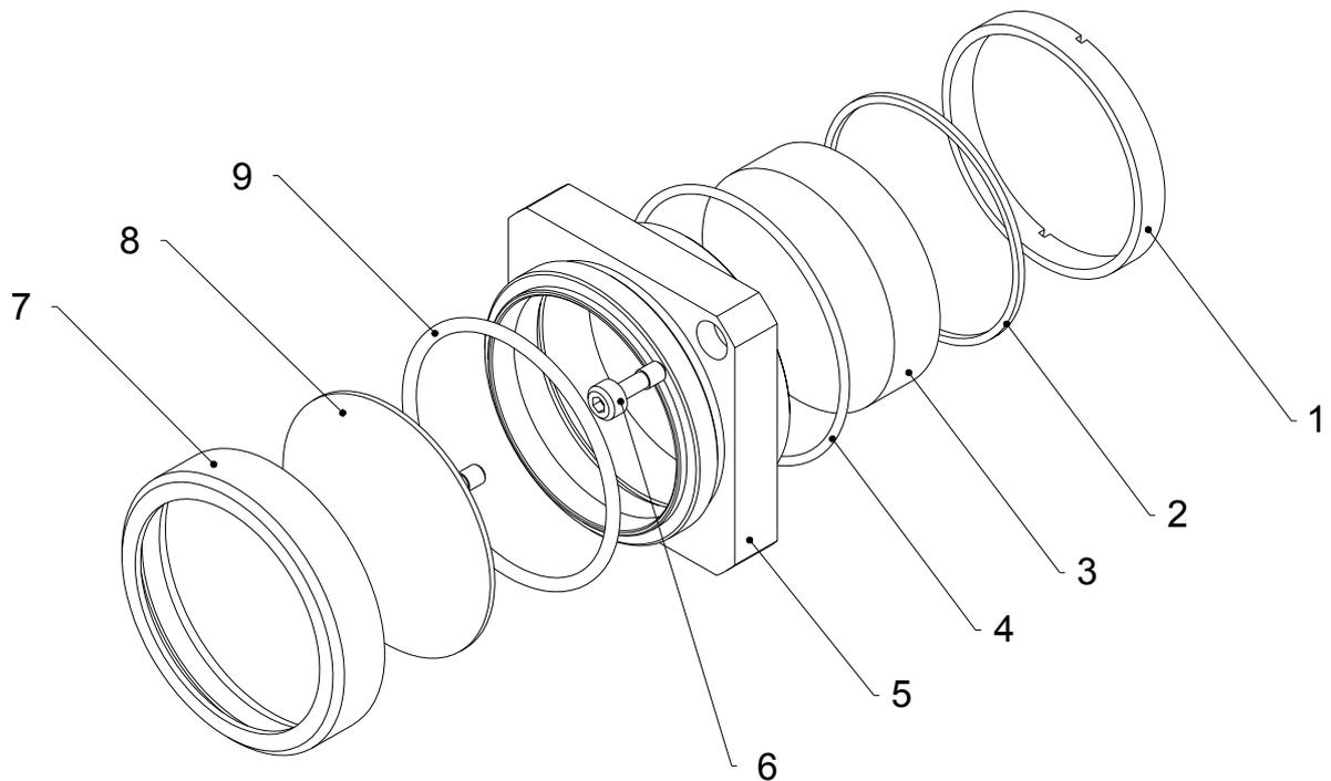
Figure 27 – Focus lens cell Removal Procedure
