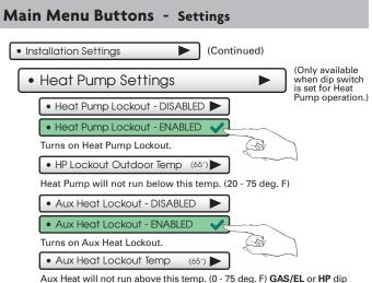
switch must be set for HP and GAS or ELEC dip switch must be set for ELEC.
