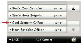
The user may adjust the ADR Cool offset. During an ADR event the cooling setpoint will be adjusted by the amount of degrees configured in this step.
