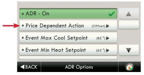
Selecting the 'Price Dependent Action' button allows the user to determine what action is taken when the price rises above the set threshold.
