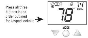
To **unlock** the keypad, press and hold the MODE button. While holding the MODE button, press the WARMER and COOLER buttons together, for two seconds.
