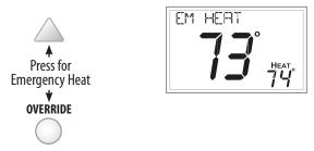
During Emergency Heat operation the thermostat will turn on the fan and the Aux strip heat when there is a demand for heat. Also during Emergency Heat, heatpump operation will be unavailable.
