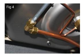
When running the pipe work to the gas locker/regulator ensure that the pipe is secured well at regular intervals or approximately 300mm. The pipe work should be grommeted or insulated as it runs through any material such as the plywood of your furniture, or metal gas box. (5)
