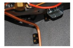
When fitting our own gas installations into the campervans we build, we use the GOK Truma regulator with mounting foot. This is a tried and tested regulator with a high-quality build. ⑦
