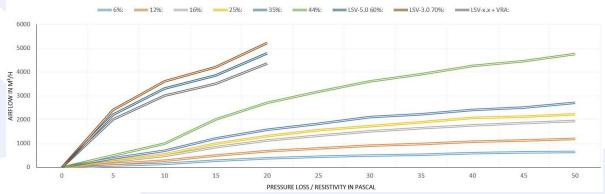
In the diagram above the airflow rates of our ventilation panels are indicated. Your installer and/or ICT company can indicate exactly which airflow rate is required. NOTE: When a raised access floor is equiped with ventilation panels without taking precautions, the fire resistance classifocation (F30, F60) does no longer apply. This is due to an open connection between the plenum (under raised floor) and the space above the raised floor and thereby the requirement for fire: oxygen.
