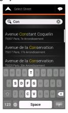
**Cause**: iGO Navigation app has a smart keyboard for address search, which means that only those buttons are active that can be used to type a name that is available on the map.
