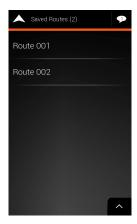
By selecting a previously saved route, iGO Navigation app recalculates the route using the saved destination and/or the waypoints.
