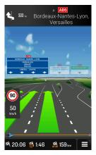
Where Provider Junction Views are not available but the necessary information exists, <u>Generic Junction Views</u> show a generic view of the junction, focusing on the number and layout of lanes only. The road signs are created from road shield, road number, and destination information received in the map data.
