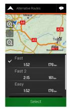
If there are suitable alternatives calculated with the route planning method that is selected in Route preferences (page 87), they are shown on top of the list. Routes with other route planning methods are shown at the bottom of the list.
