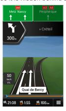
**Cause**: If you are approaching a motorway exit or a complex intersection and the needed information exists, the map is replaced with a 3D view of the junction. The lanes you need to take are displayed with arrows.
