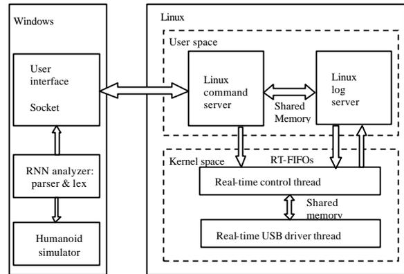
Fig. 2 Operation environment software
