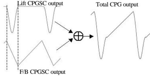
Fig. 4 Linear combination of hip pitch CPGSCs
