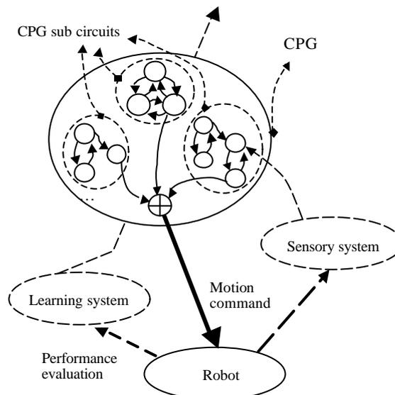
Fig. 1 Neural control mechanism using CPG
