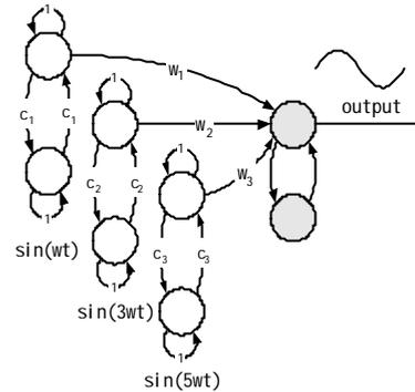
Fig. 5 Diagram for high order roll CPGSC circuit
