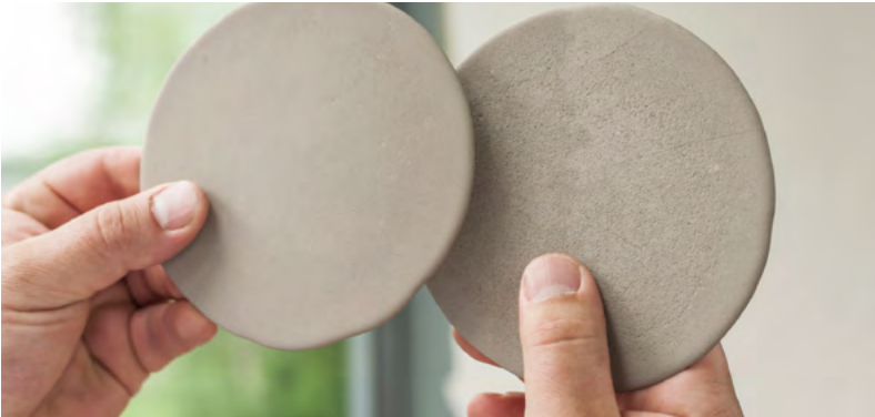
Smooth surfaces, no material build up, high surface hardness with SITREN AirVoid® 354 – Comparison: left with, right without SITREN AirVoid 354°
