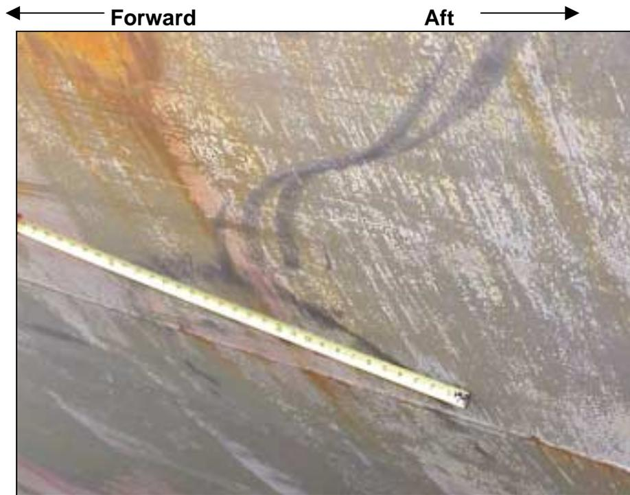
The forward most semi-circular tire mark measure 23 inches in diameter. This mark is located just under the turn of the bilge. Photo taken on October 26, 2001.
