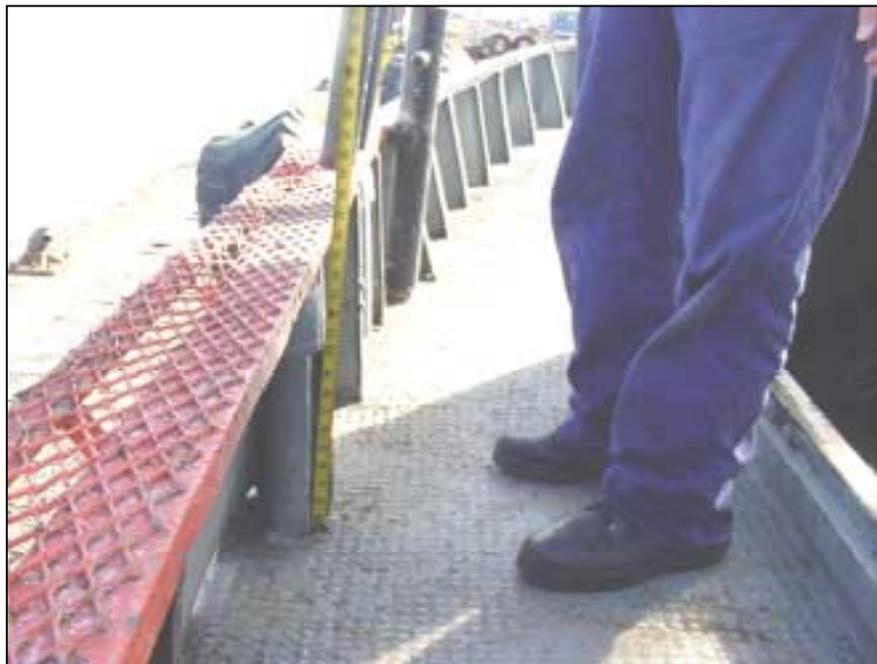
View of the port engine room vent pipe taken from port deck aft of cargo door. The vent pipe was 2" in diameter, 14.5 inches high, and situated on the outboard side of the engine room. Photo taken on November 8, 2001.
