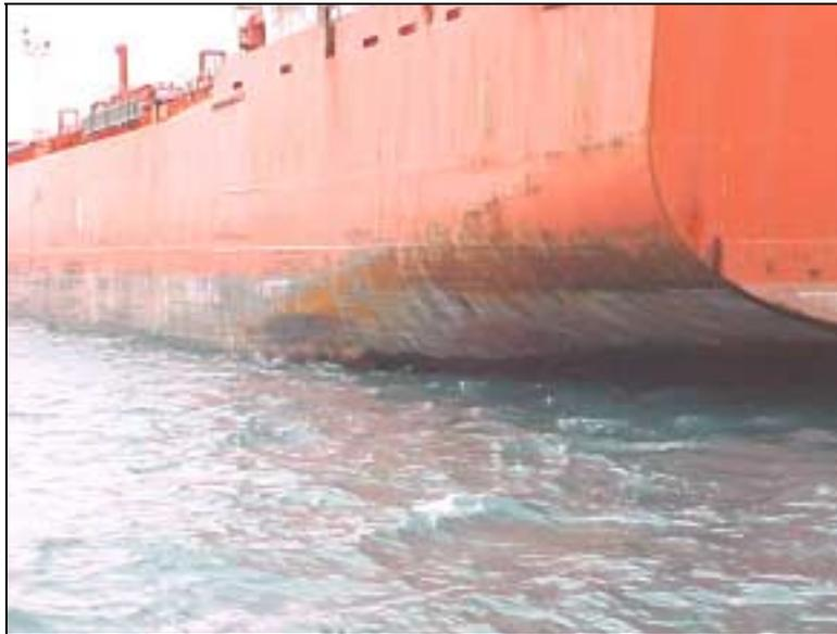
Port side SIDSEL KNUTSEN. Note the black smudge just above waterline where the turn of the bilge begins. Also note the proximity of the mark to stern. This photo was taken on October 23, 2001 at approximately 1100, 4 hours after the accident.
