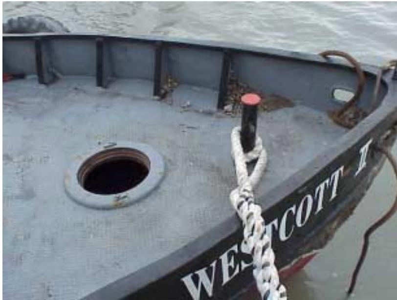
Foredeck of M/V J. W. WESTCOTT II after the vessel was recovered from the bottom of the Detroit River on October 29, 2001. Note the missing hatch cover.
