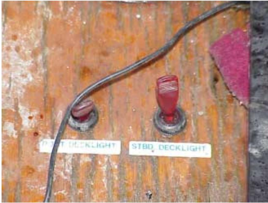
Deck light control switches on M/V/ J.W. WESTCOTT II. Port deck light switch is “off.” Starboard deck light switch is “on.” There are the normal switch positions when conducting a starboard side transfer. Photo taken on October 29, 2001.
