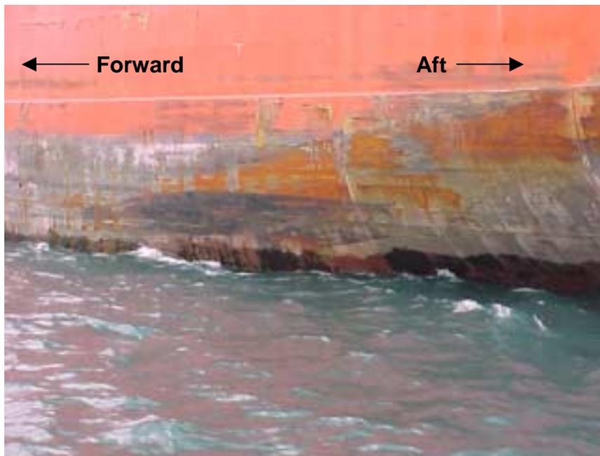
Black tire marks on SIDSEL KNUTSEN. The rust marks indicate the curvature of the hull at the turn of the bilge. Note the two semi-circular tire marks aft of the large tire mark. Photo taken on October 23, 2001.
