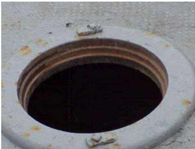
Close up of hatch on foredeck of M/V/ J. W. WESTCOTT II on October 29, 2001. The hatch measures 14" in diameter. The dogs were rusted and painted in place and were not dogged down tightly.
