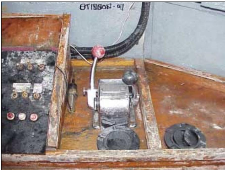
Throttle (left) and transmission (right) controls of M/V J.W. WESTCOTT II. Throttle is in “full” position. The transmission control is in between neutral and astern. Photo taken on October 29, 2001.
