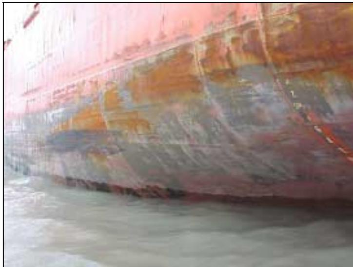
View looking forward of the black smudge marks on port side of the M/V SIDSEL KNUTSEN. These marks were created when the fender tires on the starboard side of the J. W. WESTCOTT II rubbed hard against the hull of the SIDSEL KNUTSEN. Note the semi-circular marks aft of the black tire mark. These marks appear higher than in the previous photo because this photo was taken on October 26, 2001, after the SIDSEL KNUTSEN had offloaded some of its cargo.
