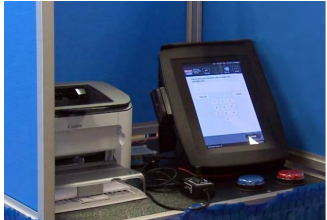
The ImageCast X pictured here with joystick and paddle button accessible voting devices.
