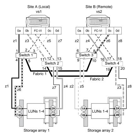
In the sample illustration, four array LUNs are allocated on each storage array for the MetroCluster configuration. LUNs of equal size are provisioned on the storage arrays at both sites, which is a SyncMirror requirement. Each FC initiator port on each V-Series system has a path to each V-Series LUN on the storage arrays. The ports on the storage array are redundant, and are configured as follows:
