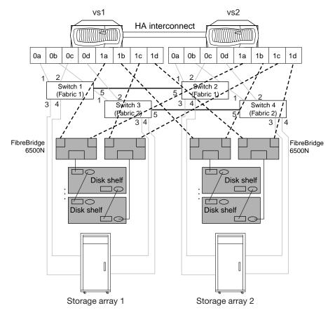
As the illustration shows, the stretch MetroCluster uses direct FC connections between the V-Series systems and the FibreBridge 6500N bridges. Eight FC initiator ports are required on each V-Series system, four for the FibreBridge 6500N bridges and four for the connections to the storage array via the switches.
