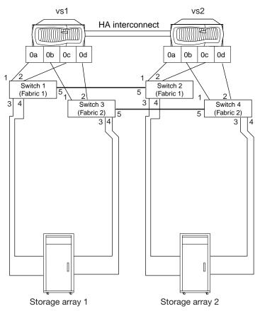
The following block diagram shows the connectivity when FibreBridge 6500N bridges and disk shelves are added to the stretch MetroCluster configuration from the previous illustration. The connections for accessing array LUNs are purposely grayed out to make it easier for you to see the connections for the FibreBridge bridges.
