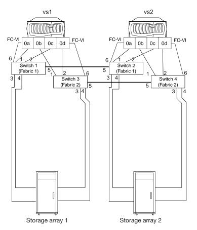
The following block diagram shows the same fabric-attached MetroCluster, but with disks as well. Notice that the same switches are used for access to the storage arrays and the FibreBridge 6500N bridges, but different switch ports are used for the bridges and the storage arrays. Also notice that different FC initiator ports are used for the two types of storage.
