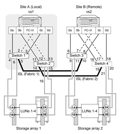
**Note:** A port pair consists of two FC initiator ports that are used to access the same set of array LUNs. For example, V-Series FC initiators 0a and 0d are accessing the same LUNs. See the *V*-*Series Installation Requirements and Reference Guide* for specific information about port pairs for your platform.
