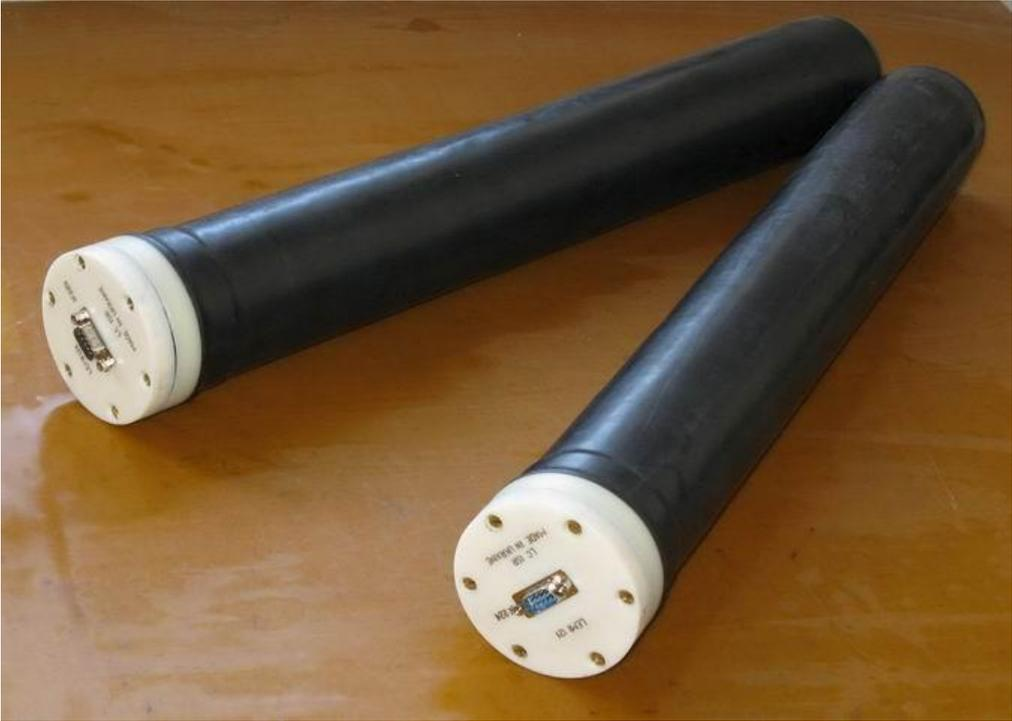
Induction sensors (also known as search coils), because of their measuring principle, are dedicated to varying magnetic field measurement.
