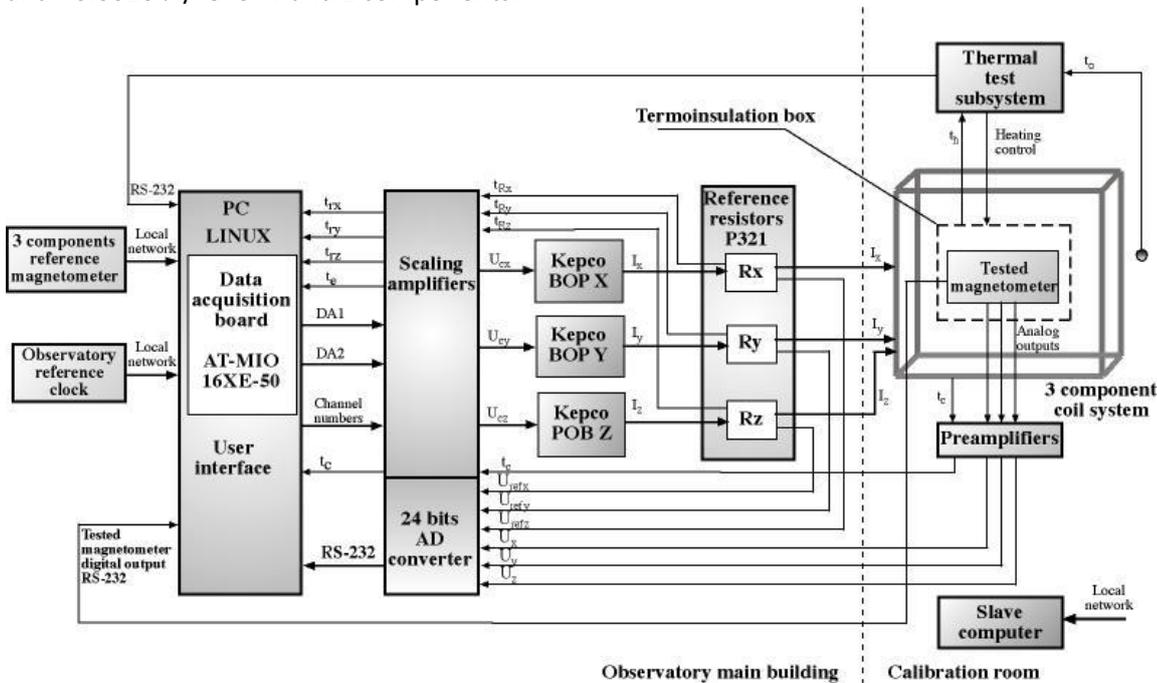
Fig. 3. Functional diagram of the magnetometer calibration system.
