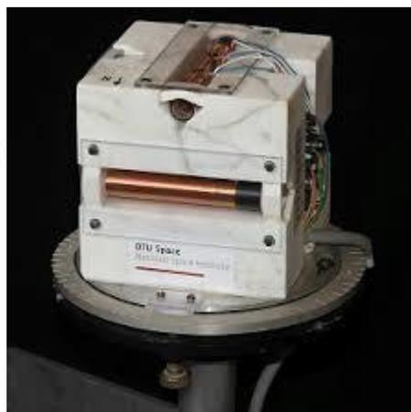
On the left is a ring-core sensor which has lower noise than the bar type. On the right is the sensor made by the Danish Meteorological Institute. Here the sensing elements are set in a marble cube and compensating coils are wound around the fluxgate sensors.
