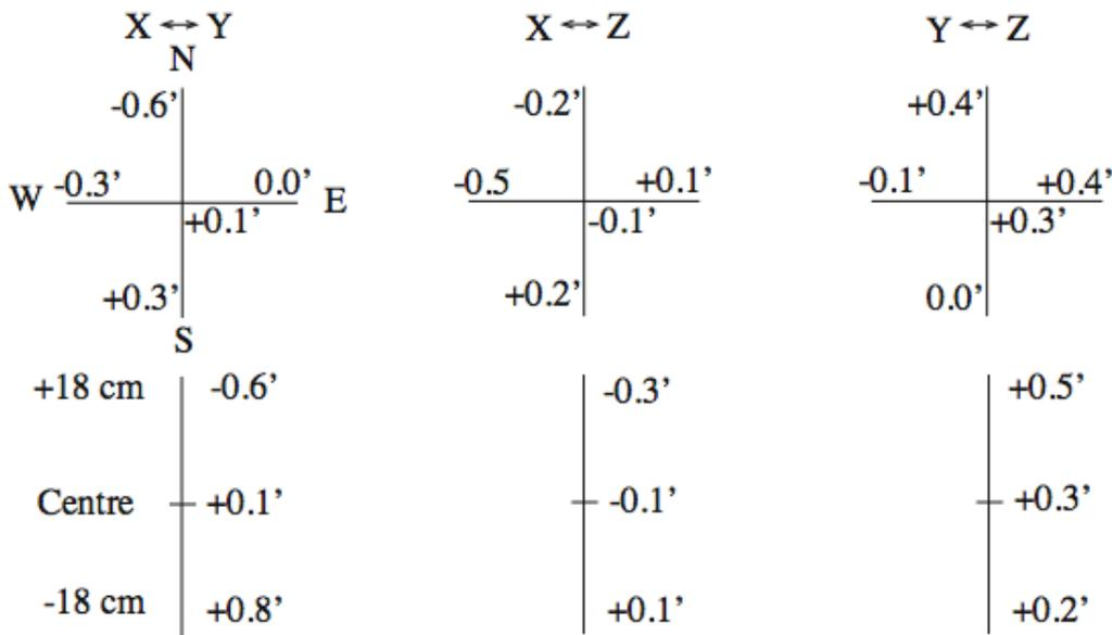
Fig. 2. Angle errors between the orthogonal magnetic fields in the center of the coil system and 15 cm to north, east, south and west (above) and 18 cm above and below the center (below).
