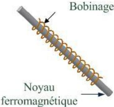
Induction sensor constituting with a winding (orange) surrounding a ferromagnetic core.
