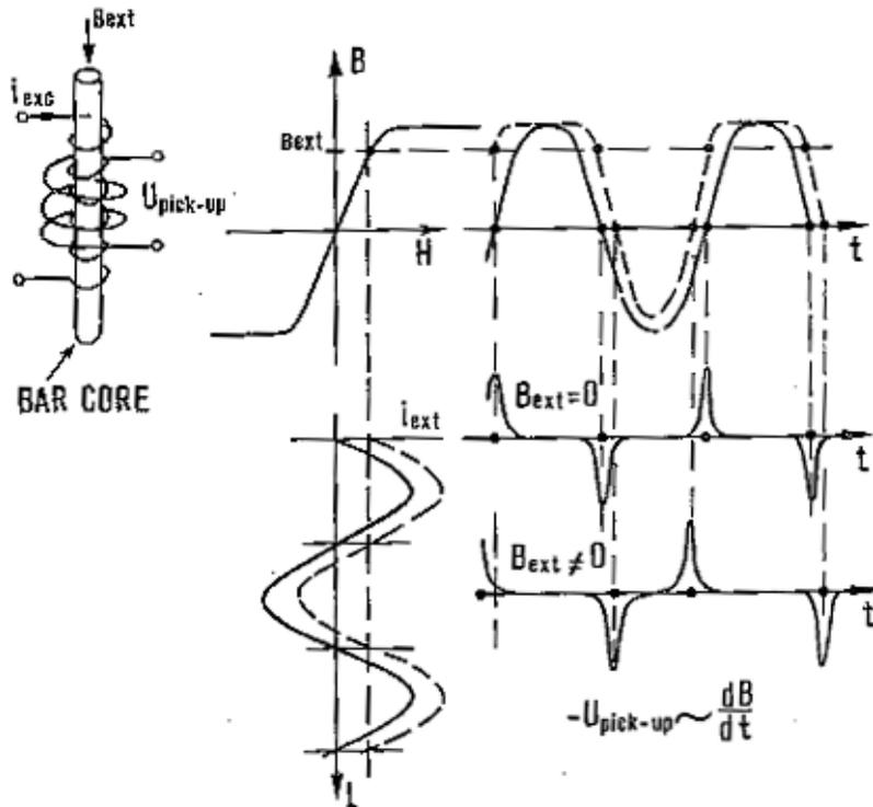
Two coils are wound around a ferromagnetic core. An alternating current is fed to the primary coil. If an external magnetic field is present the induced field is limited to one direction by the hysteresis of the core material. The difference between the inducing and the induced fields gives a signal that can be observed. The signal is observed with the pick-up coil.
