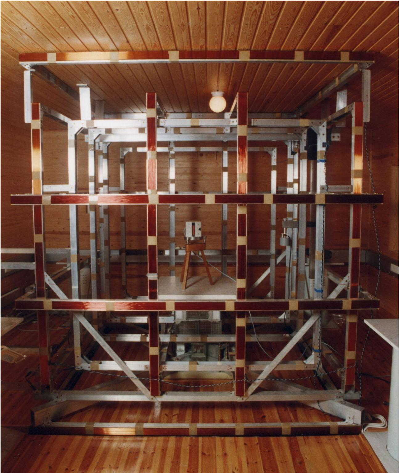
Fig. 1: Calibration coil system of the Nurmijärvi Geophysical Observatory.
