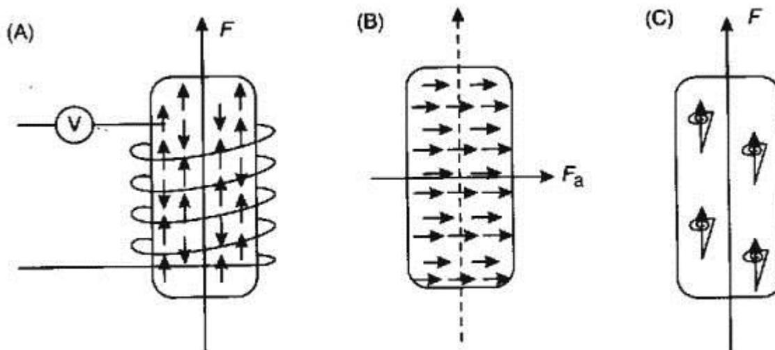
A proton magnetometer measure the total magnetic field strength and is not very sensitive to direction.
