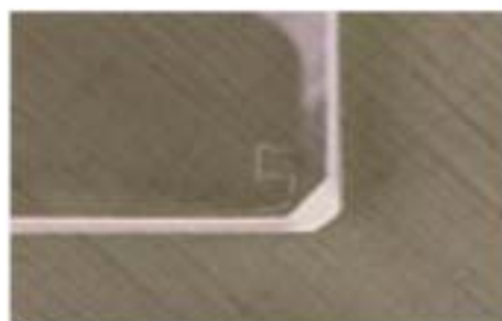
Borofloat plate etched as Grade 5.
