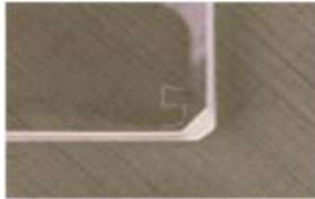
Borofloat plate etched as Grade 5.
