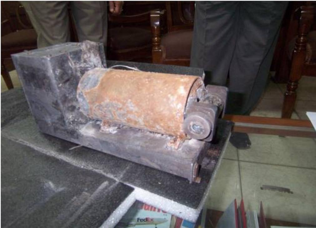
**Photo 6: Damaged CVR Recovered From the Crash Site**
