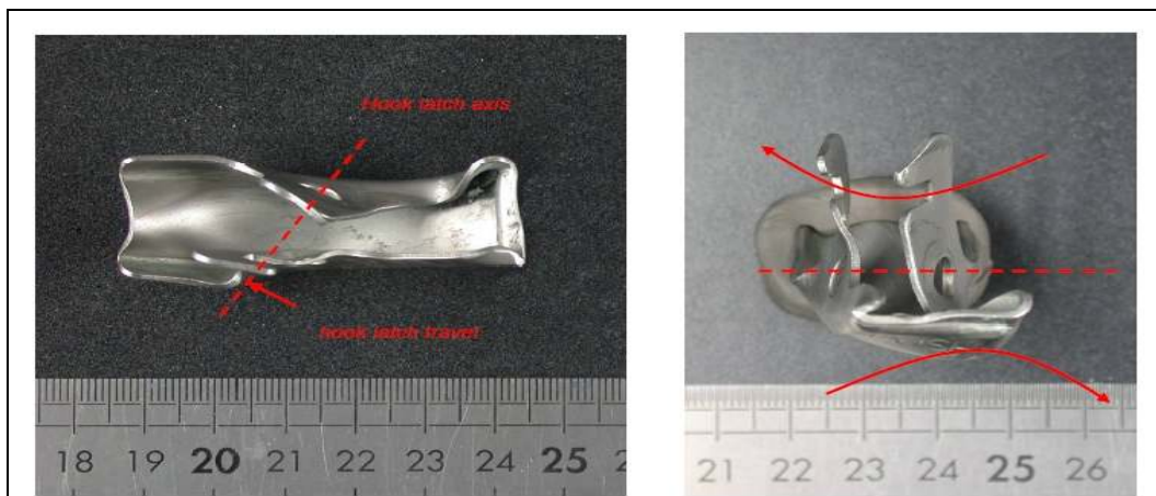
[Picture 22] Deformation of Pushbutton
