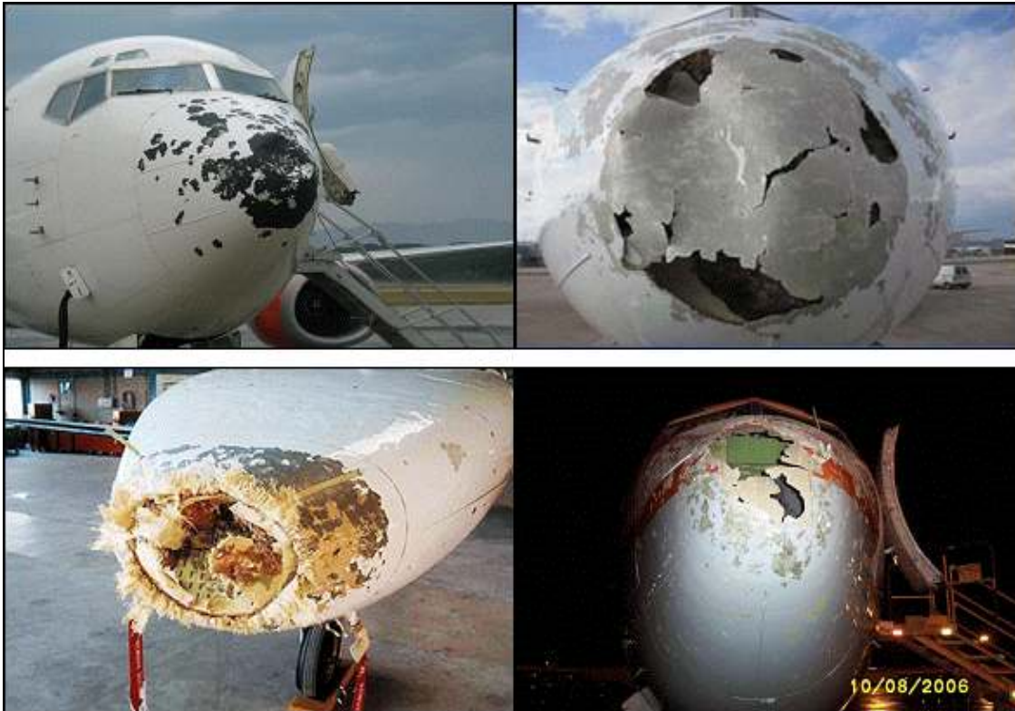
[Picture 18] Shape of Damage to the Front Radome Due to Hailstorm
