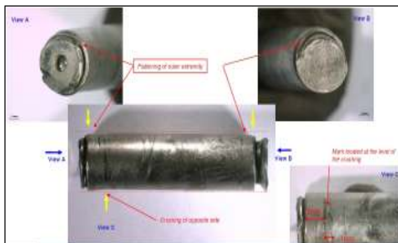
[Picture 24] Damage to Pushbutton Axle
