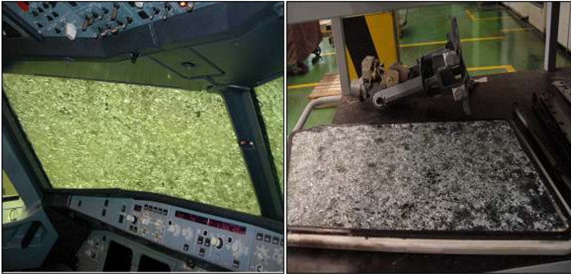
[Picture 13] Damaged Windshield Installed in Aircraft (Left) and After Separation (Right)
