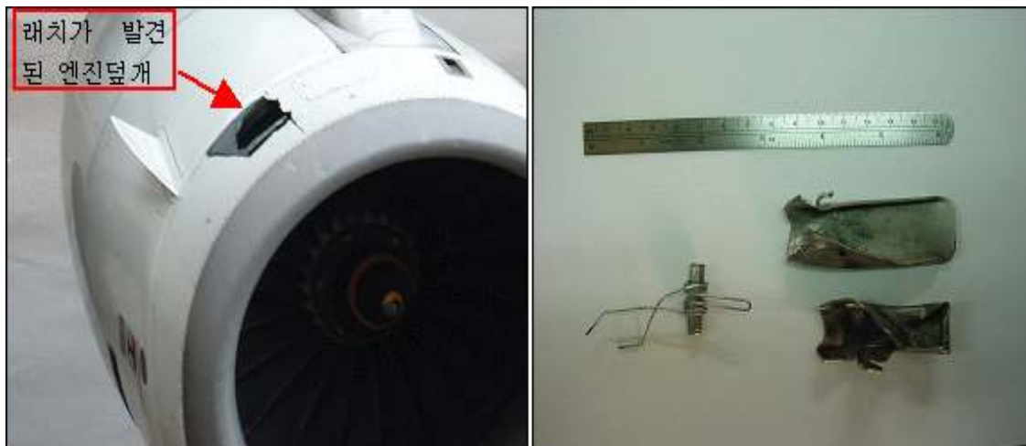
[Picture 15] Cowl of No. 1 Engine Where Latch was Found and Damaged Latch
