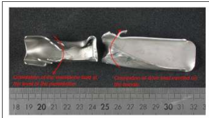
[Picture 23] Damage to the Left Handle and the Pushbutton
