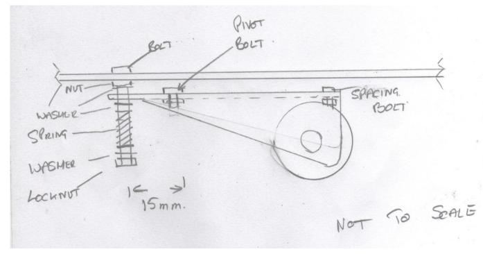
pony truck were supplied by him and were of sufficient length to contain the spring. The bolt is drawn longer than was in practice the case - see the picture below, which shows that it was more or less level with the centre line of the rear driving axle.
