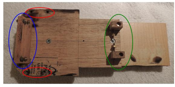
As you see, this is the jig after use. The red ellipses each sit over 2 holes drilled in the jig through which the bottom end of the handrails were pushed. The bracket at the back (circled blue) was used to bolt the back of the cab to the jig and was made from an off-cut of
