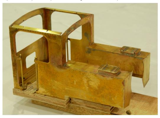
that I had not taken the 45 degree cut off the back of the jig at this point - I only recognised the need for this later in the build.
