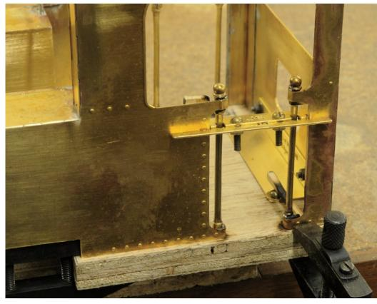
Also visible in this view is the bracket supplied with the etched parts used to secure the cab to rear of the the footplate. There came a point when I was moving the assembled cab on and off the rest of the loco and needed this bracket on the This was loco. when I made (and over engineered) a bracket from hardwood which I attached to the jig. Before finally moving the bracket designed for securing body to
