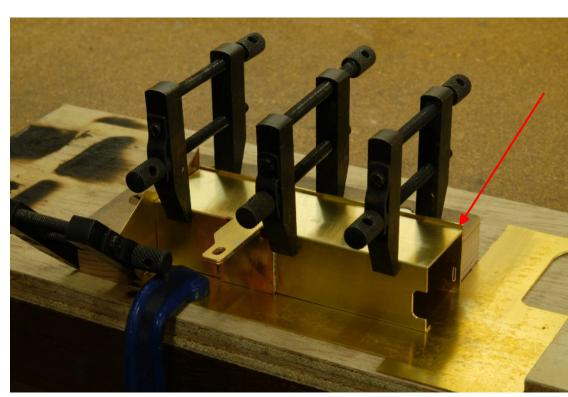
the tank cab assembly in the first place: I heated the assembly until locally dull pink and applied the solder, at which point is ran readily. The jig and clamps prevented the other parts becomina unsoldered but found that providing I used a short and narrow flame, heating was reasonably localised.
