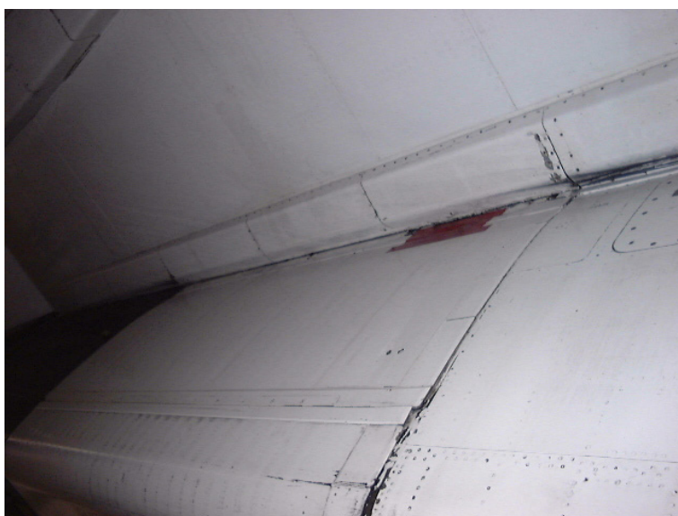
Figure 65: In red, the lateral air conditioning air bleed door used for the air conditioning
