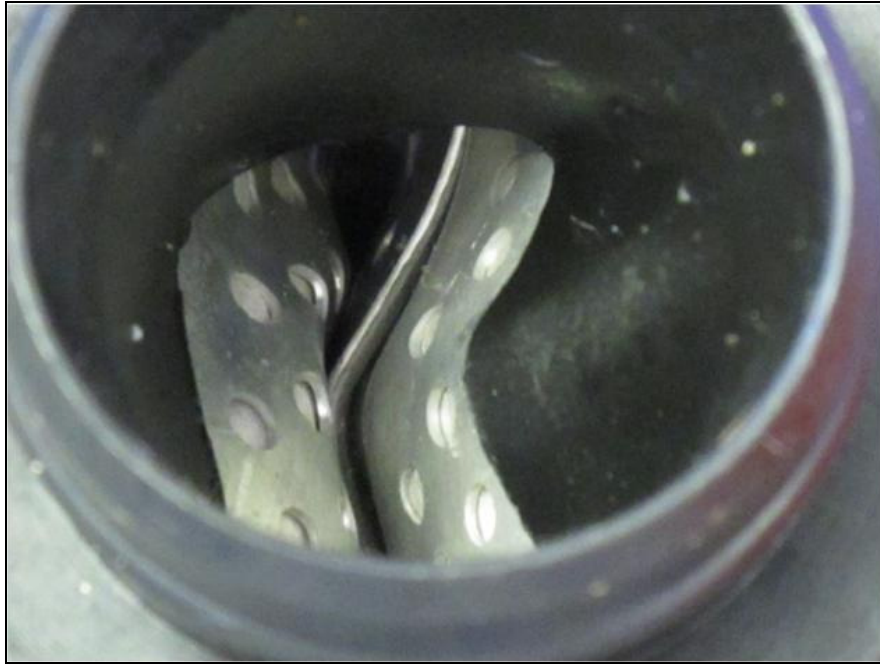
Figure 46: The centre aluminium core tube of the collapsed filter monitor was crushed
