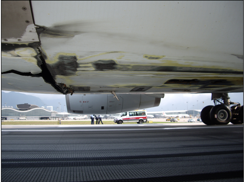
Figure 19: Damage on No. 1 engine cowl lower surface
