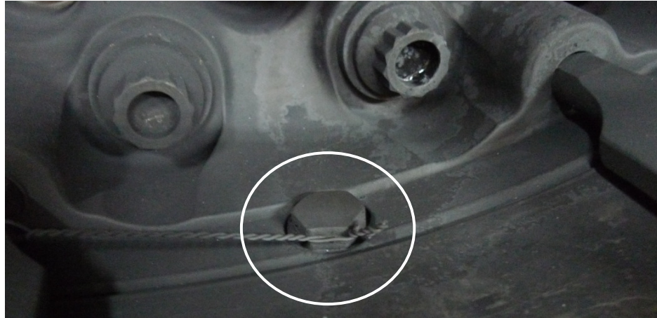
Figure 49: One event fusible plug installed to the wheel showing the centre core was intact
