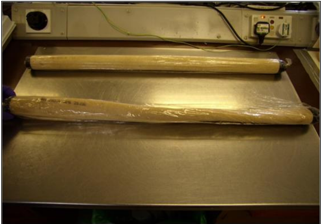
Figure 45: The collapsed Batch 2 filter monitor placed adjacent to a normal filter monitor
