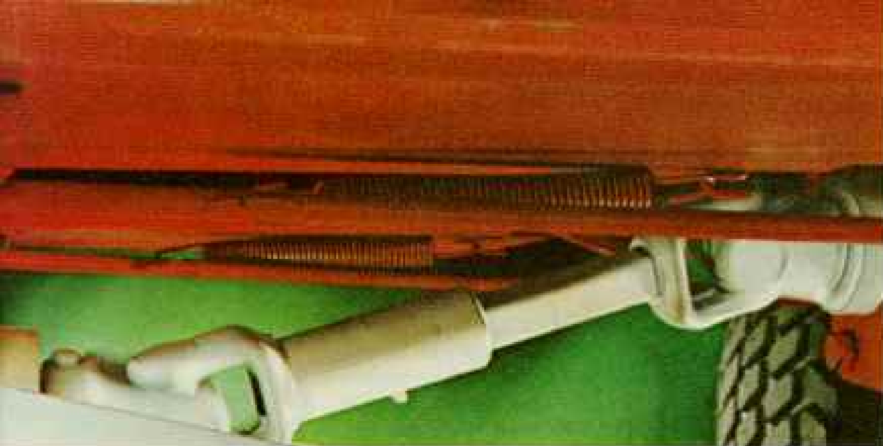
The reliability of unique all-gear drive—no belts to slip, break or adjust
