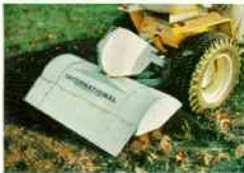
Rotary tiller—7-in. depth, 32 to 38 in. wide.
