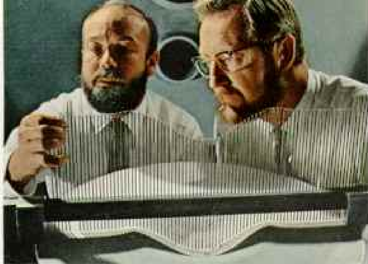
DONALD E. GAULT , right, and William L. Quaide, experts on craters, adjust rods that register contours of a man-made crater at NASA's Ames Research Center near San Francisco. An aeronautical engineer, Mr. Gault has developed a gun that hurls projectiles up to 28,000 feet a second to simulate meteorites, aiding study of crater formation.
