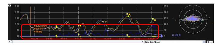
For drag racing, there is one more analyzing type. You can divide the laps into four or ten segments. And the duration of every segment will show on the screen.
