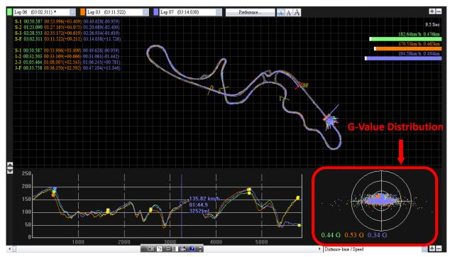
Show Brake line: It can show you the braking line on the track. You can compare the tracks and get acceleration and braking information. (The thick lines present the braking zone, and the thinner lines present the acceleration zone.)
