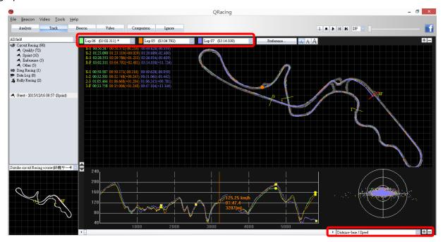
Select by **Time-base** will show the fastest and slowest speed difference line on the graph when doing multiple lap comparison.
