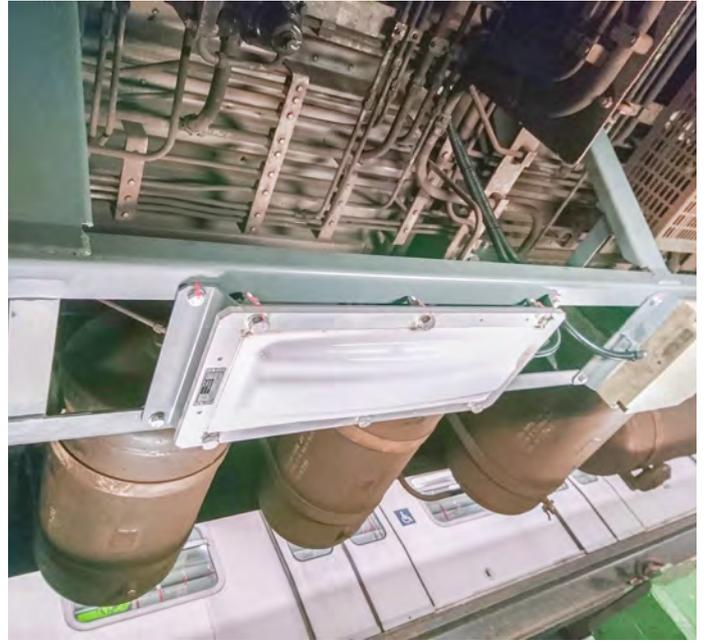
Train fitment. Left, additional operator's display in existing cab. Right, CBTC underframe interrogator transponder added.
