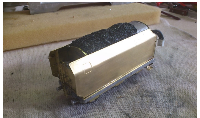
Above: After considerable adaption the brass tender body is ready for attachment to the boiler assembly.
