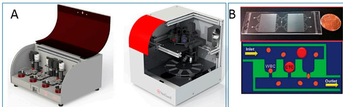
**Figure 2.** The “Celsee” system, able to process blood samples and perform image analysis (A). Microfluidic setup and scheme of the mechanism of CTCs capturing with inlet and outlet for pumping blood samples and reagents through the device (B). Modified with permission from [59].
