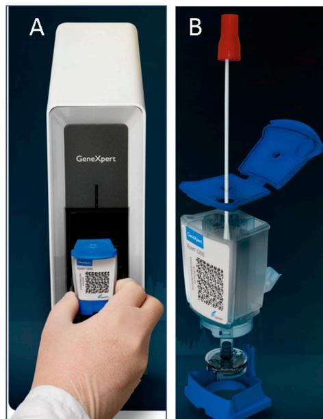
**Figure 10.** The Cepheid GeneXpert portable platform for qPCR. (A) The GeneXpert I model, including a single module able to run one cartridge at a time. (B) Exploded view of the disposable GeneXpert cartridge. The upper, bigger part includes the processing chambers where sample preparation occurs. Behind them (on the right in the picture) is the reaction tube where qPCR takes place. Below the processing chambers is the valve body, which drives all the fluidics. Figure modified from [93].
