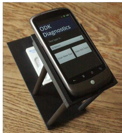
Figure 3: Low-cost 3D-printed platform used to capture images of RDTs.
