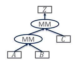
void kernel 0(float \*A, float \*B, float \*C, float \*Z) { if (idx < 1024) buffer[idx] = MatMul f(A, B); Global Sync(); Z[idx] = MatMul f(buffer, C); h[idx] = temp1;
