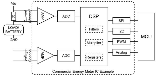
Figure 4: Architecture of a typical energy metering circuit.
