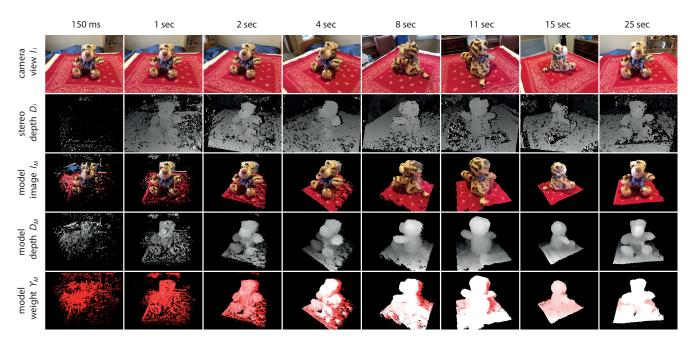
Fig. 5. Progress of object scanning from a sequence of length 25 seconds. Each column captures live camera view, per frame depth map, raytraced RGB, 3D model and model confidence, over time.
