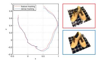
Fig. 3. Camera pose estimation based on feature-based tracking (red) and dense tracking (blue) together with resulting models. Dense tracking increases robustness in situations without salient image features visible at all times.
