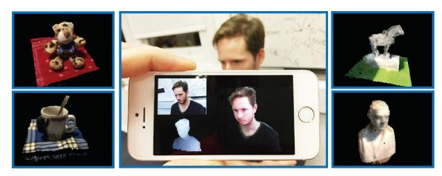
Fig. 1. Example objects scanned in real-time on a mobile phone using our system. Note we only use the internal RGB camera, and all computation is performed on the device.
