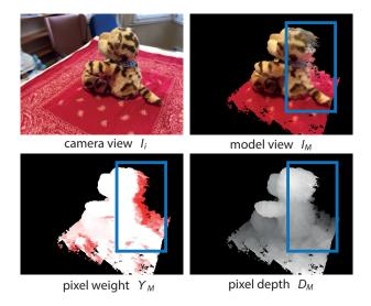
Fig. 4. Detail of the weighted image alignment scheme for camera tracking. Model view  $\{I_M, D_M\}$  is used for per-pixel alignment of camera image Ii. We downweight pixels corresponding to noisy parts of the model using the projection  $\Upsilon_M$  of weights W(p) stored in the TSDF.
