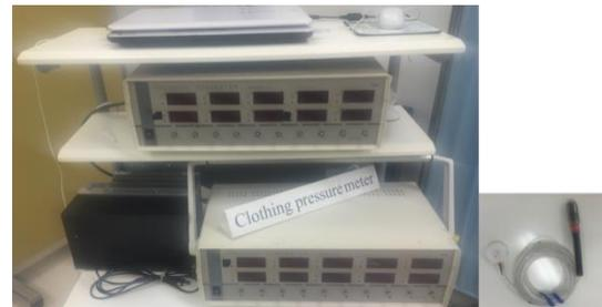
Fig.4.2 AMI3037-10 for measuring clothing pressure
