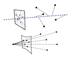
Figure 1: Two-step approach for radial distortion absolute pose. First, using radial alignment constraints we estimate the pose of the camera up to an unknown translation along the principal axis (blue line). Using the full projection equations we then solve for the remaining translational degree of freedom jointly with focal length and distortion parameters.
