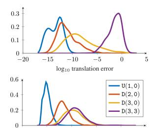
Figure 2: Solver stability on synthetic data. *Top:* Rootbracketing with Sturm chains (Section 4.1.1). *Bottom:* Polynomial eigenvalue formulation (Section 4.1.2).
