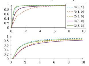
Figure 5: Cumulative histogram over the median reprojection errors (in pixels) for the densely sampled grid points (c.f. Figure 4). *Top:* Using ground truth poses (except for  $t_3$ ). *Bottom:* Using estimated camera poses (Section 3.2).
