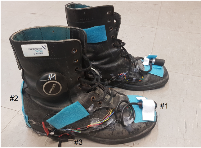
Fig. 1. The first version of the system: "These boots were made for walking..." yet, the electronics embedded into them were highly sensitive and the measurements were noisy. The system is composed from the following components: #1 a ranging device, #2 few IR-LED targets, #3 Micro-controller with 10 DoF sensors, #4 a GNSS device for testing: compering the approximated path with the Ground Truth (GT).
