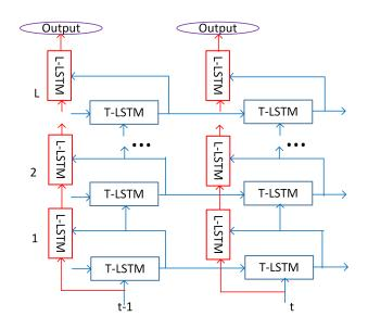
Figure 2: Flowchart of layer trajectory LSTM (LT-LSTM). Layer-LSTM (L-LSTM) is used to scan the outputs of time-LSTM (T-LSTM) across all layers at the current time step to get summarized layer trajectory information for senone classification. There is no time recurrence for L-LSTM. Time recurrence only exists between T-LSTMs at different time steps.
