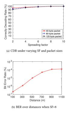
Figure 5: Determining spreading factor
