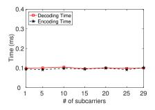
Figure 14: Encoding and decoding time at BS
