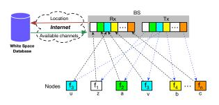
Figure 7: SNOW architecture with dual radio BS & subcarriers
