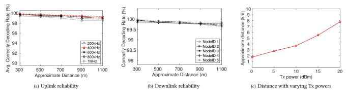
Figure 9: Reliability over distances and varying Tx power.
