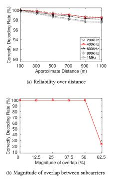
Figure 6: Determining subcarriers
