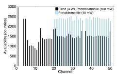
Figure 1: White space in the US counties [58]: showing the number of counties (y-axis) where the channels (x-axis) are white space.
