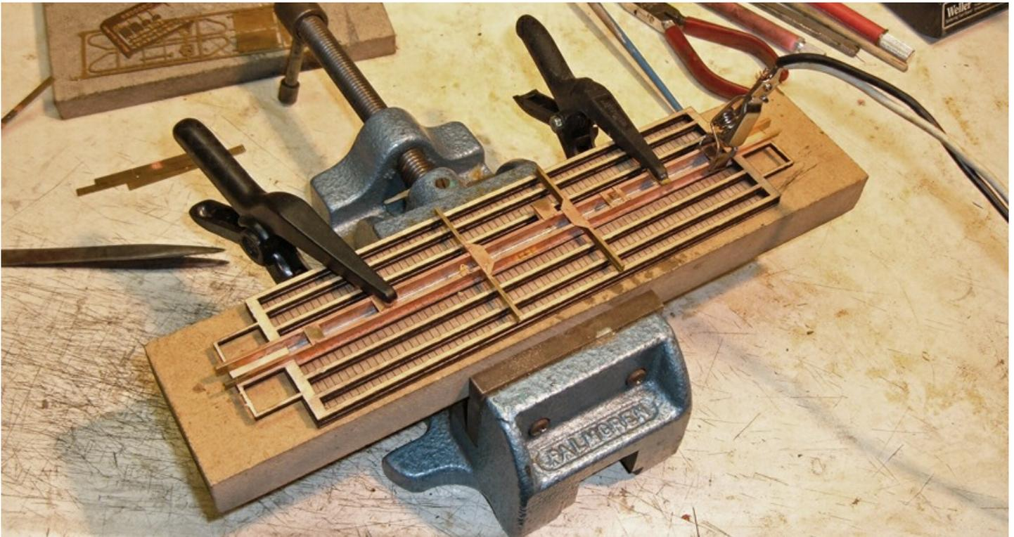
*This was my first attempt at a work table. I needed a way to hold the model flat while I assembled the frame. This was tried because I needed to hold the model flat and keep the stiff wire from the resistance soldering rig from dragging the model to where the wire wanted to be, which was never where I wanted the model to be. This worked well, but the thick table made from the 3/4" particle board limited the clamps I could use.*
