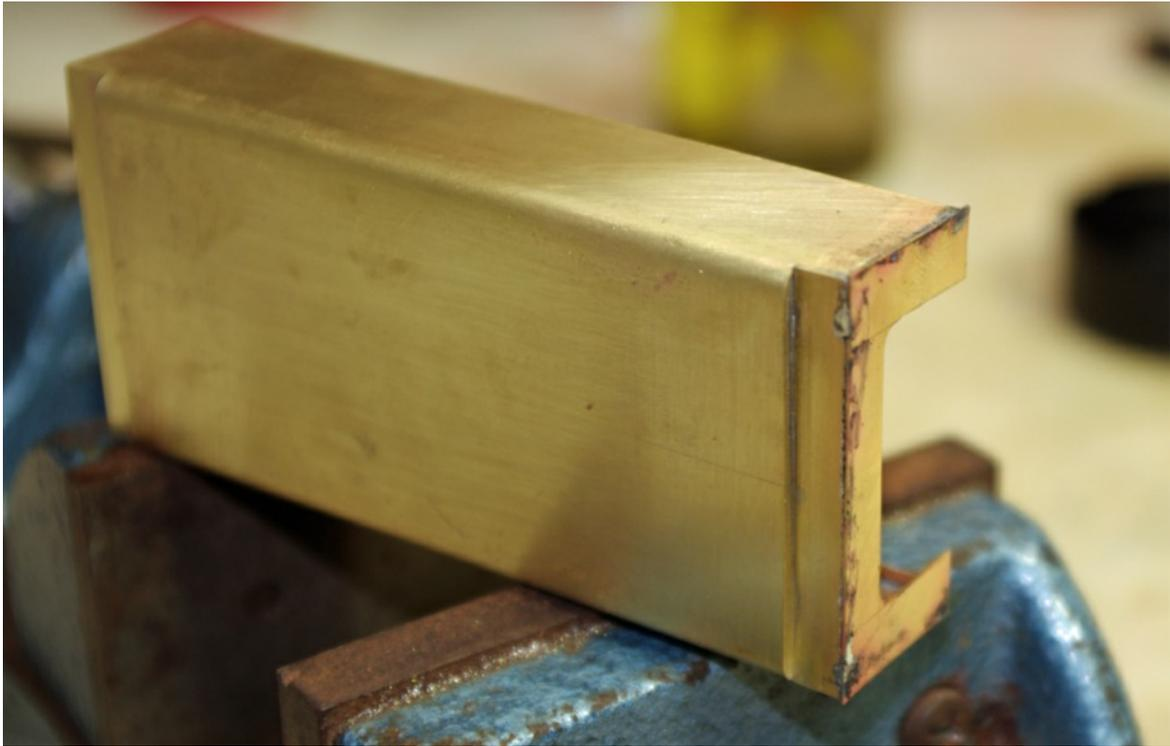
*This is how the tank looked after soldering the ends on. All that remains now is to file the sides flush.*
