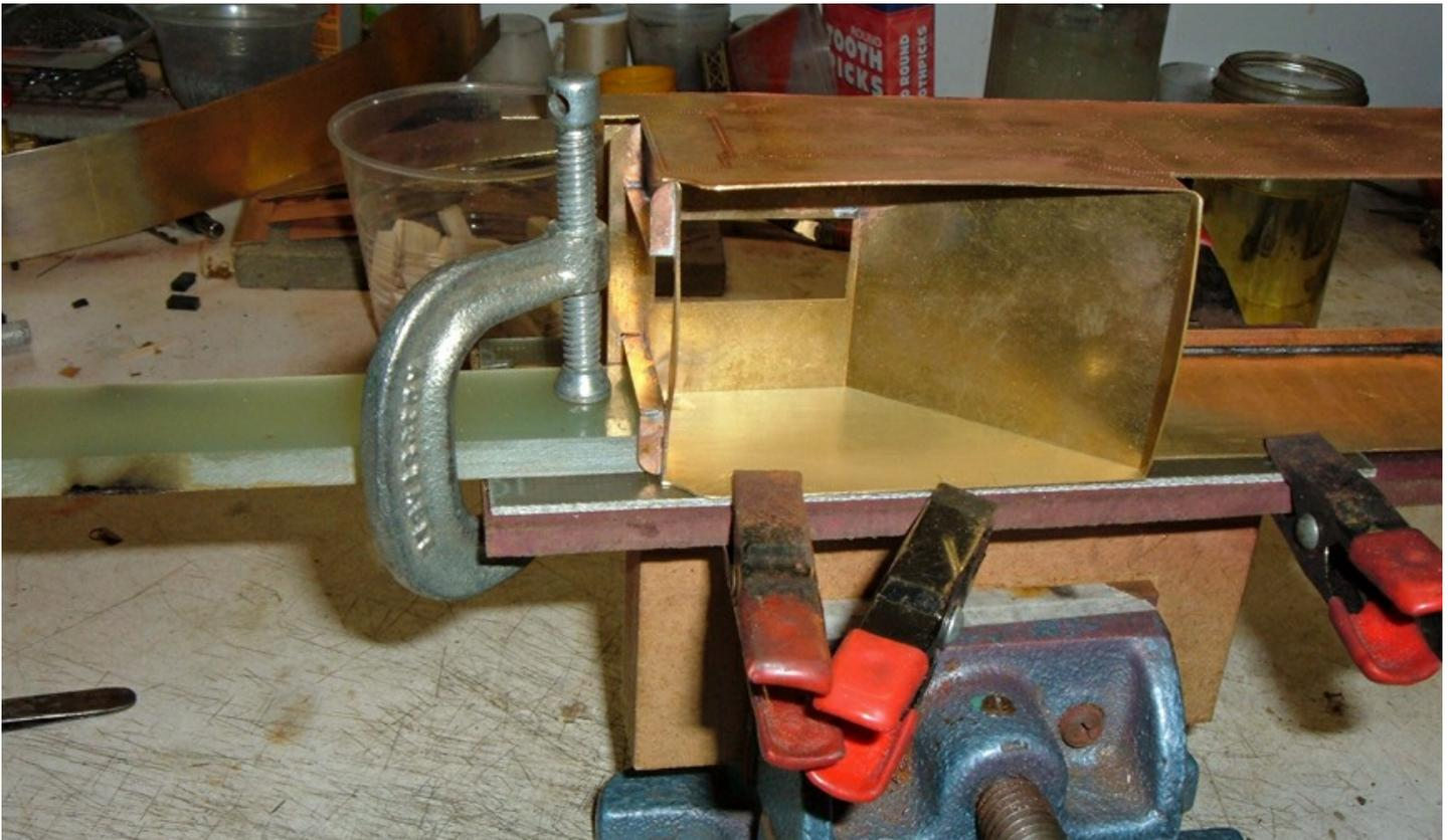
*This is an S Scale tender I was working on. Notice I put a piece of circuit board material between the model and the work table. The bar under the "C" clamp is a piece of Garlite plastic that is similar to the circuit board material. Notice how it is charred from a previous project. It would not smoke like the wood, but still melted and it is expensive. This was not going to work.*
