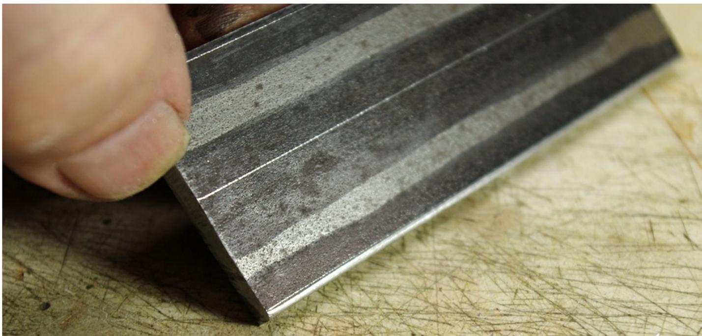
Here you can see the scribe marks better. Notice I have scribed marks close to the edge. These marks are the radius of the bend or .048" in this case. I used these marks to file the radius on my form. See the explanation below for how to do this.
