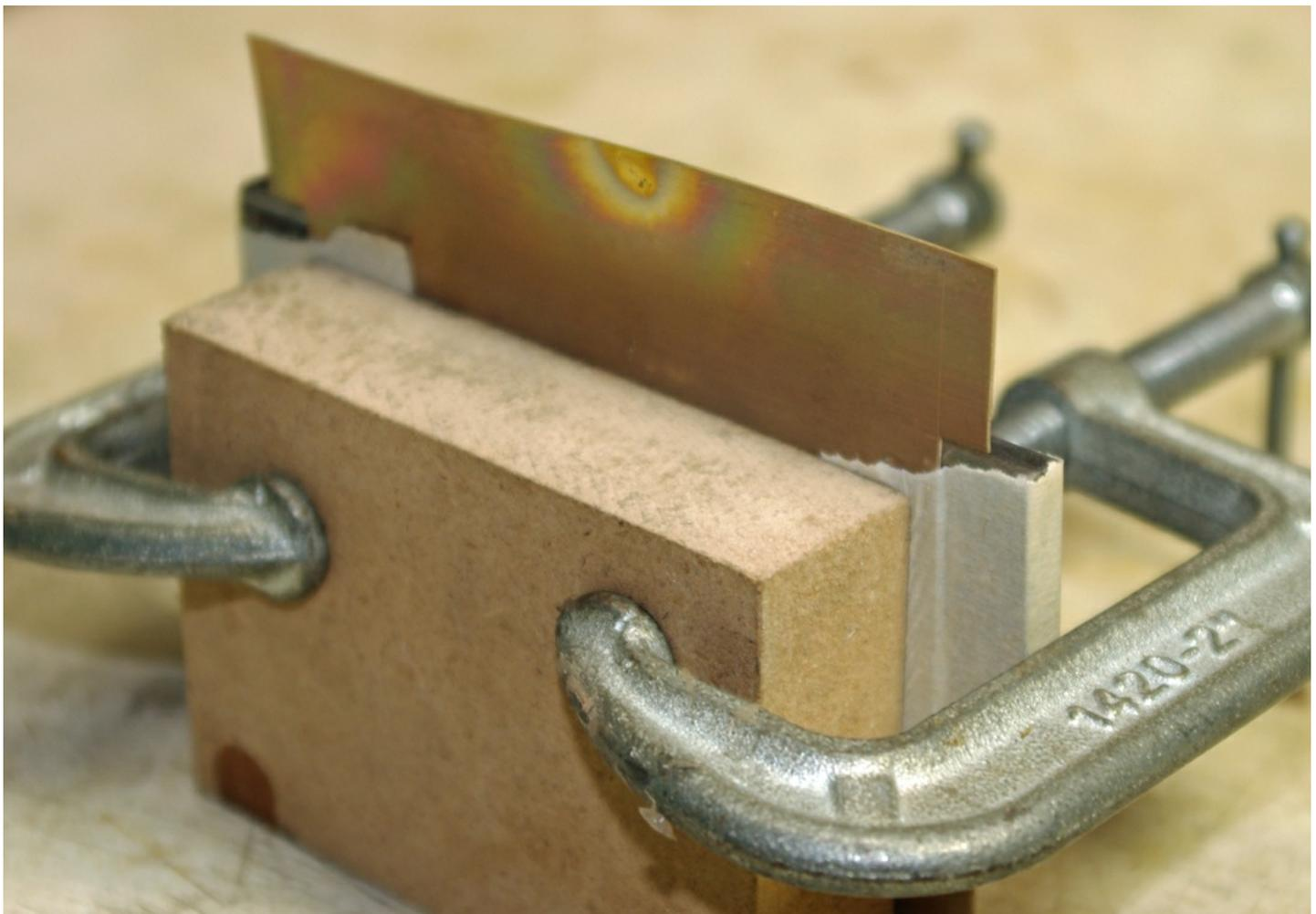
*I positioned the wrapper on the form and taped it in place. Then I clamped a block of wood on it, as shown, to hold it tight in place. Make sure the wood is just short of the edge. Next, I bent the wrapper over the form by placing the wrapper at the edge of a block of wood and rolling it over to follow the form.*
