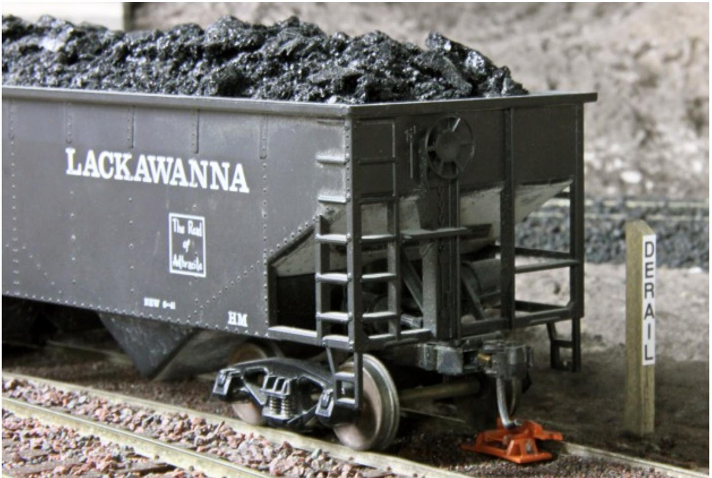
*Properly installed derail located on the upper mine runaround track.*
