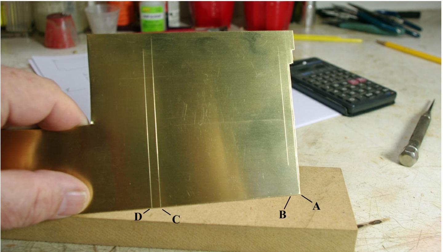
*Here I have laid out the vertical lines. Notice that I drew a vertical line over on the far right. This establishes a square edge on the right. It also establishes point A from the sketch. Measure along the bottom edge and scratch small marks. Then, use your square and scribe to scratch in the vertical lines.*
