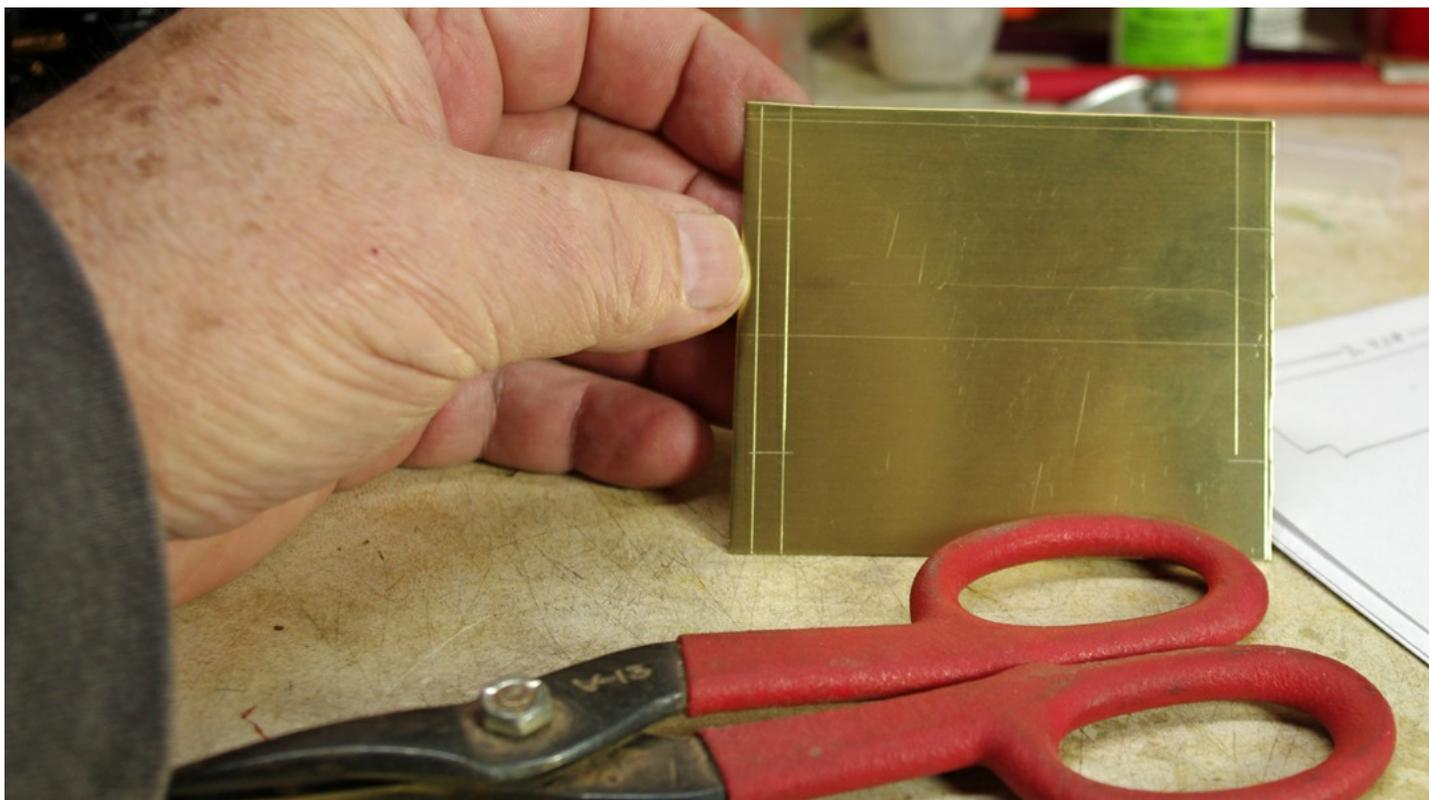
*In this view, I rough cut the sheet using the metal shears. Don't try to cut to the line. The shear tends to curl the brass when it cuts. I have had better results by cutting close and filing the edge flat to the line with a #2 cut mill file.*
