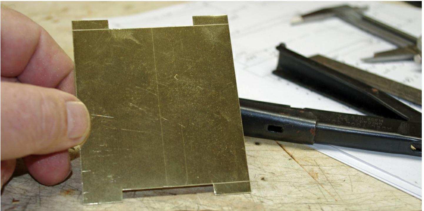
*This is my tank wrapper after I finished cutting it out. The nibbler will cut very close to the line, but I still left a little and finished with a file.*
