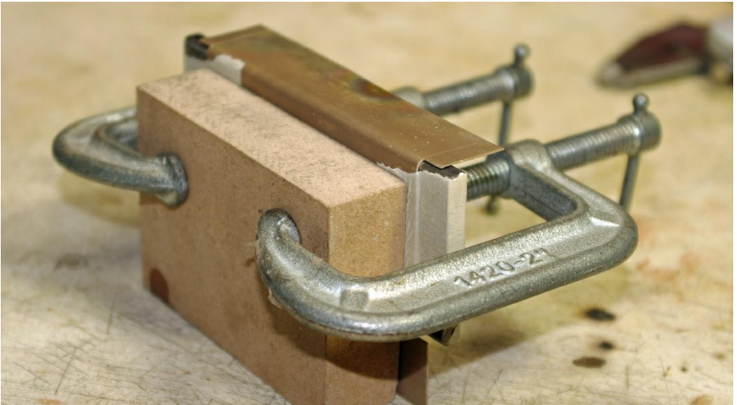
*This is how the wrapper looks with one side bent over. Notice how nice the bend looks. Also notice how there is no springback on the brass. This is because I annealed the brass first. Brass work hardens and now that I have bent it, it is getting hard again.*
