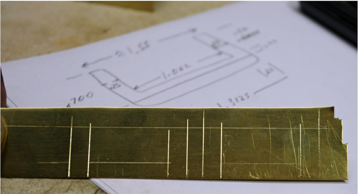
*Now it was time to lay out the ends of the tank. This model has the older single tower drive, and I needed to make room for the drive shaft to go through the tank. I have two of them laid out here. Do the layout the same way you did the tank wrapper.*
