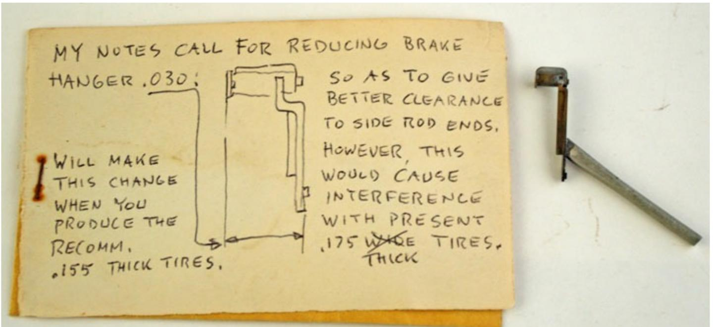
*This note was attached to this pattern for a driver brake hanger. Herman is telling Bob Smith from Central Locomotive Works that this part will need to be changed when they change the thickness of the tires. The .175" thick tire was the old NMRA standard. Today the standard is .147".*
