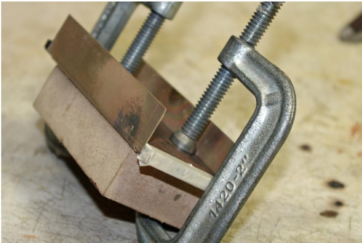
*After I had the first side bent, I repositioned the wood block and bent the other side over. Notice that the two sides of the tank are parallel and the tops are the same. Using the form, and making sure I positioned the wrapper with a center line, made this all work out. Again, by annealing the brass I did not have to fight the springback, and the bend came out where I wanted it.*
