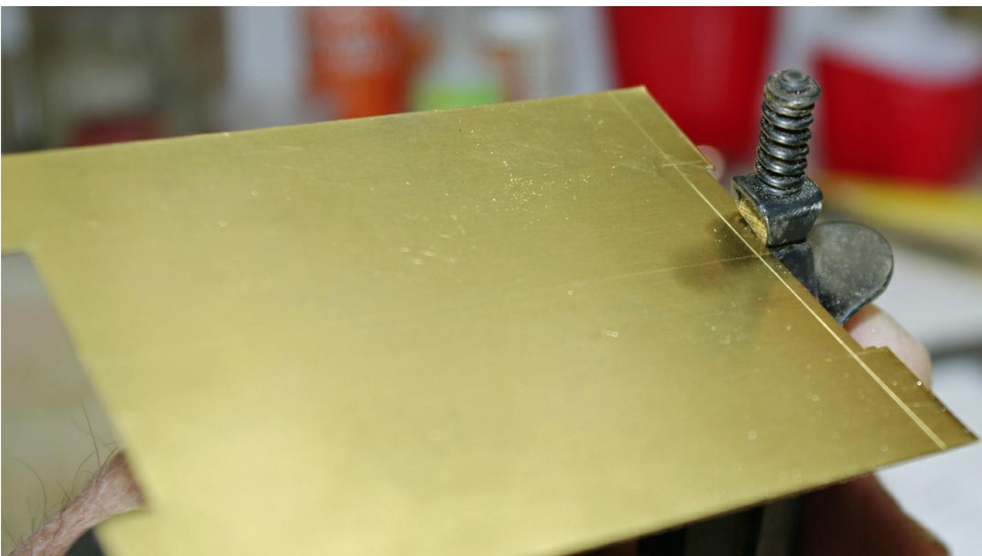
*You probably noticed that there is a notch in the tank. It would be hard to cut this inside corner with the shears, so I used a nibbler. These are available from tool suppliers and are handy gadgets. I have also used mine on styrene with good results. They nibble little bits out of the sheet, and make nice sharp corners.*
