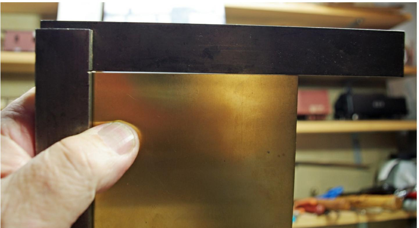
*When doing layout work, you never want to work from two edges and here is why. Notice that even the factory cut edge is not square. Never assume the material you are working with is square.*
