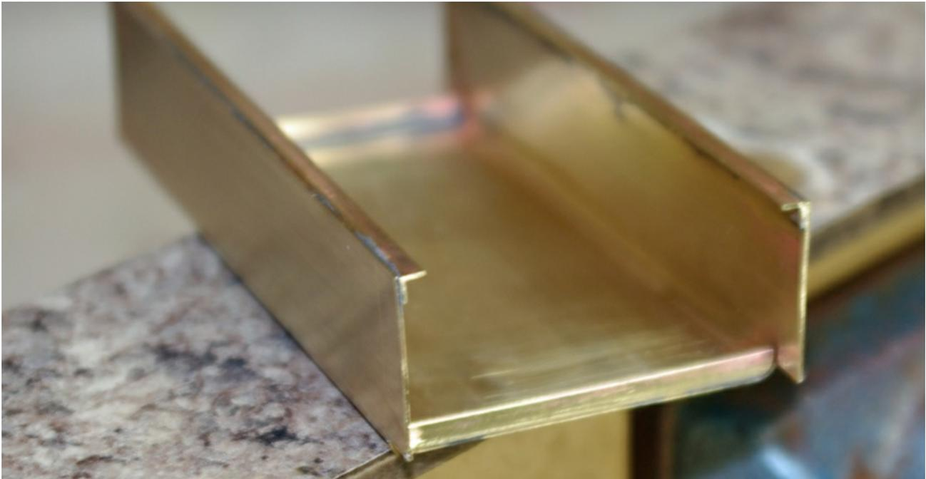
*After the top edges were done, I needed to do the step. I used a piece of the 3/32" angle again. I fitted it to length and filed the corners round to match the tank. Then, I clamped it like I did the top edge and soldered it in place. This straightened out the bottom of the tank, added some strength, and also made the face of the step.*
