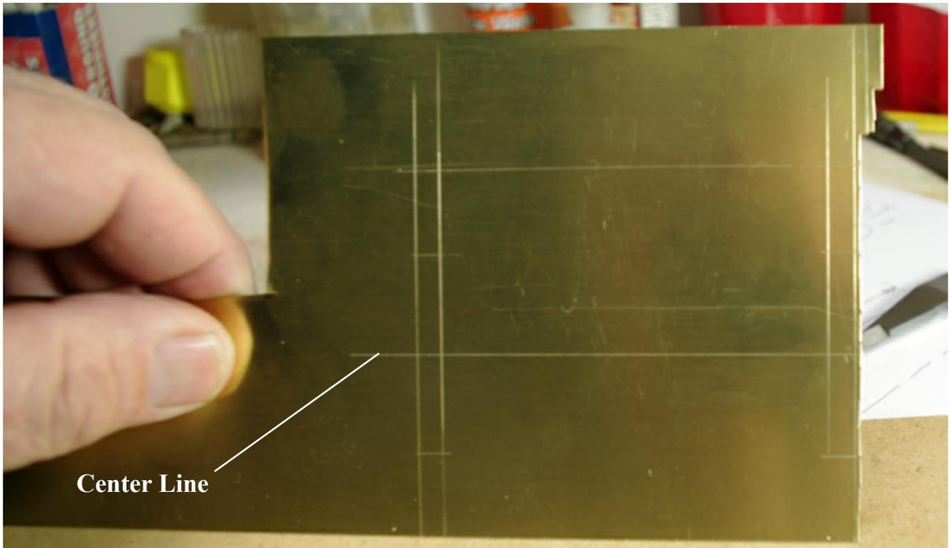
*In this view, I measured up from the bottom of the sheet to get the horizontal lines. I scribed them using the tip of the caliper. This is not good practice, but works in many cases. There is error put in because you can not keep the caliper square to the edge and it is hard on the tip of the caliper. The proper way is to set your adjustable square and run it along the bottom edge with your scribe following the square.*
