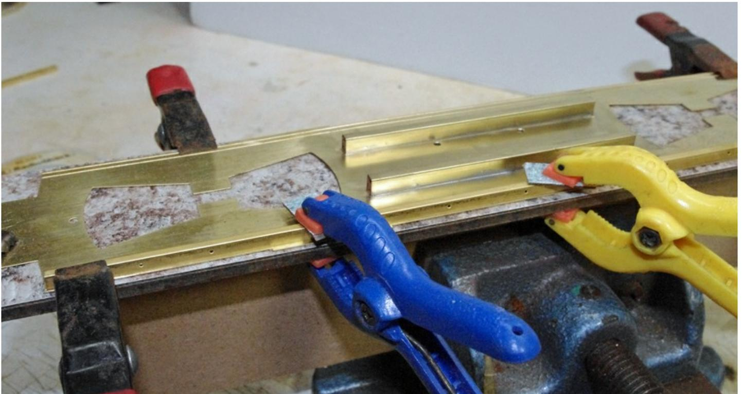
*This is an S Scale Alco RS 1 frame and some recent work. Notice the small pieces of countertop laminate between the plastic clamps and the work. This was just enough insulation that the plastic clamps did not melt. Also, I have glued a piece of countertop laminate to the work table top. The set up is working very well.*
