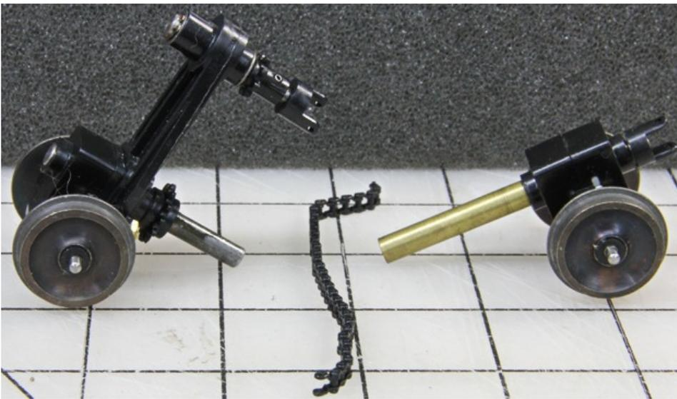
With the sideframes off, you can simply pull the two wheel assemblies apart.
