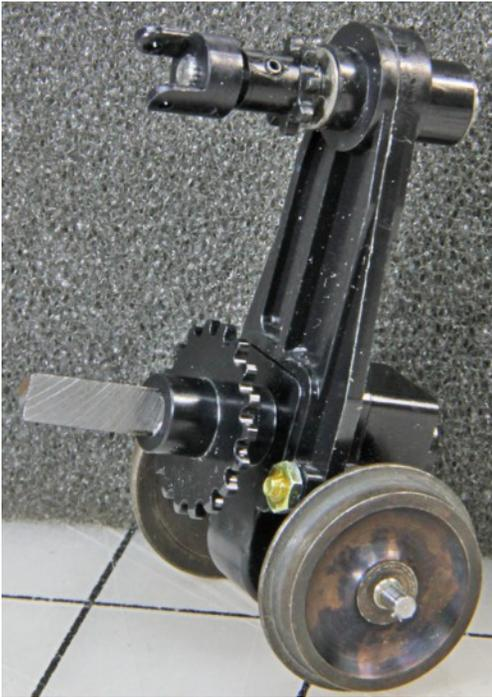
Push the new gear on the shaft and eyeball the alignment so that the chain will be lined up with the upper gear. You can make a minor adjustment after the chain is back on.
