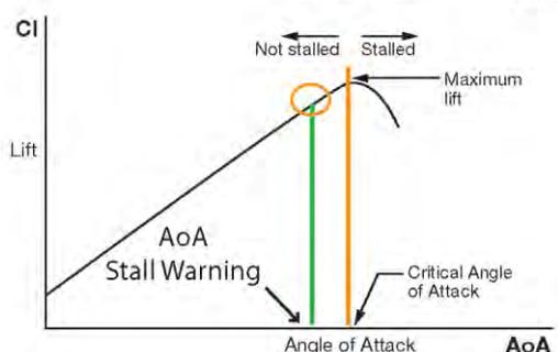
The EFCS adjusts the AoA MAX limitation to account for the reduction of the AoA STALL with increasing Mach number.
