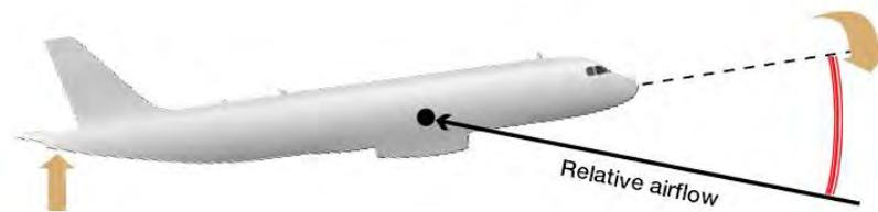
Figure 3 Pitch control is a direct AOA command
