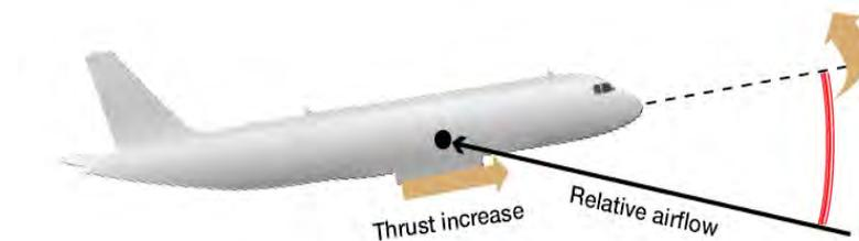
Figure 4 Adding thrust leads to an increase in AOA
