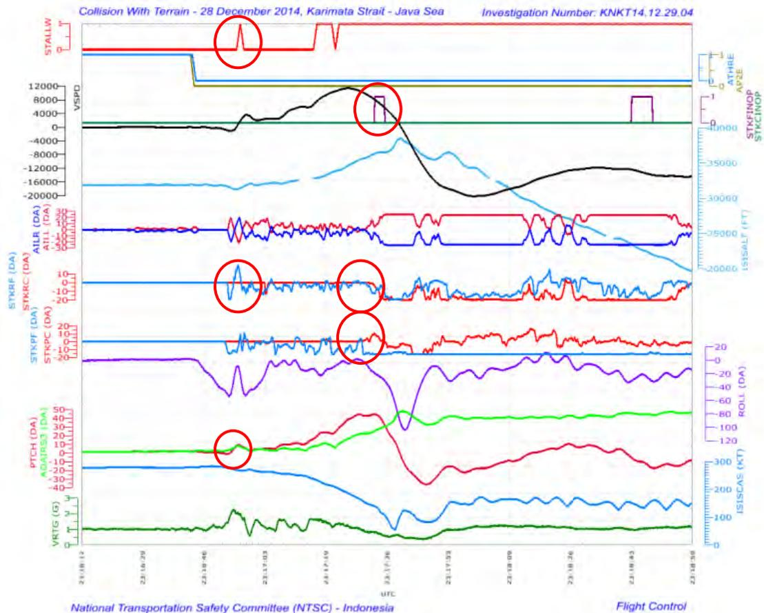
**Figure 22: Pilots inputs on side stick**
