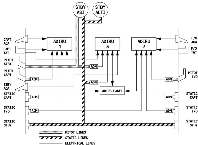
**Figure 13: line probes schematic**
