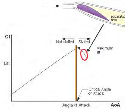
When the AoA reaches the value of the maximum CL, the airflow starts to separate.
