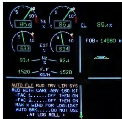
**Figure 34: The ECAM messages after RTLTLU 1 and 2 fault**
