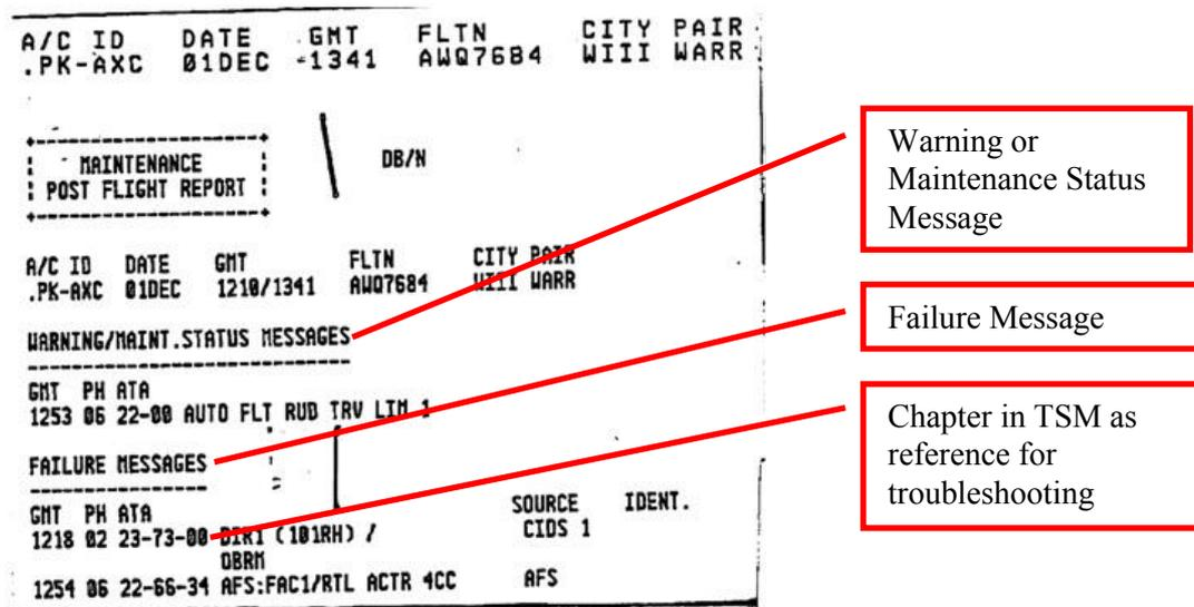
Figure 6: Typical Printed Post Flight Report (PFR)
