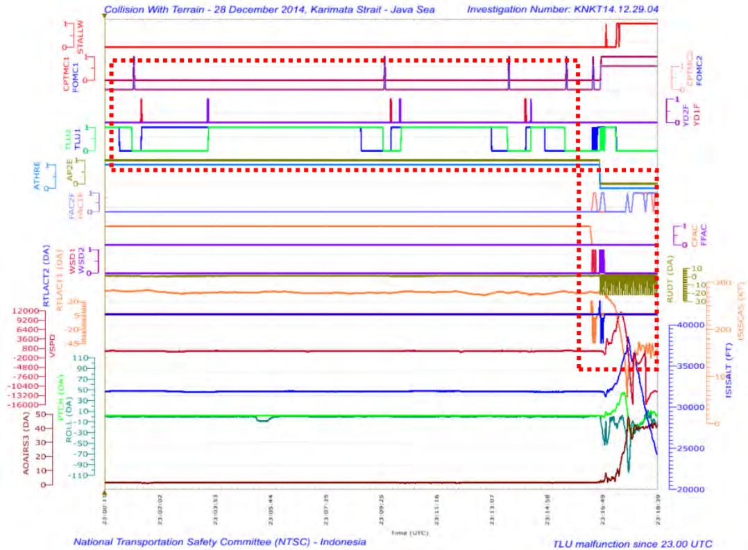
**Figure 20: RTLU problems and pilot actions**
