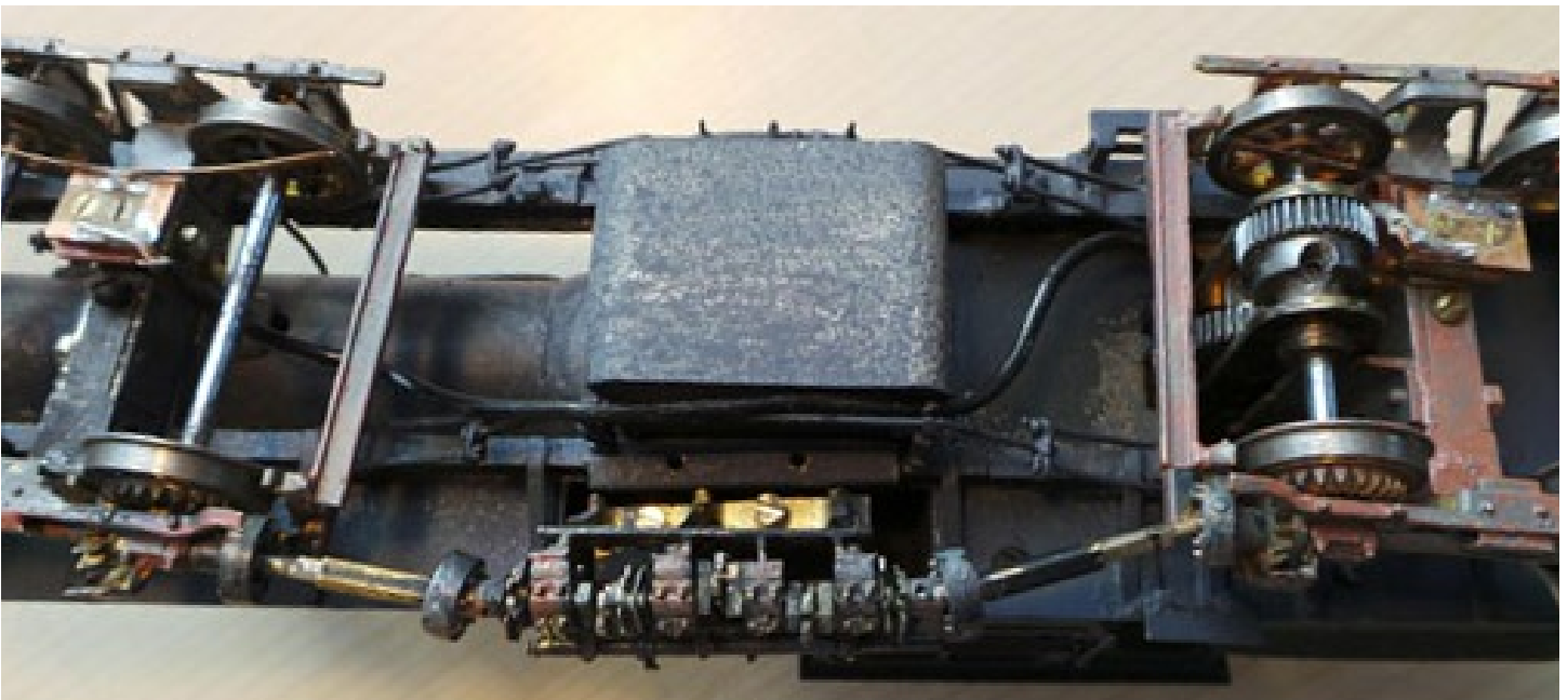
This photo shows the underneath details of my completed model, and how the cylinder block can be unscrewed from the chassis. It also shows tiny screw heads retaining the crankshaft and the ends of the universal joints have small holes drilled in the bearing. (Tim)
