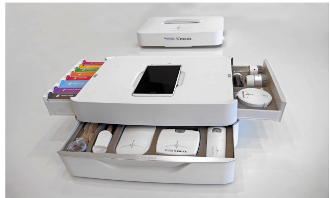
Figure 1: DeepQ Tricorder. DeepQ consists of four compartments. On the top is an HTC mobile phone, which acts as a data hub and also runs the symptom checker. The drawer on the right-hand-side contains optical sense. The drawer on the lower-front contains vital sense and breath sense. The left-hand-side drawer contains blood/urine sense.
